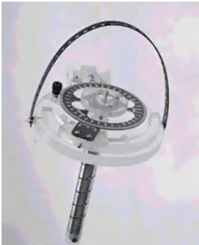
Figure 3: Spiral contractometer for measuring internal stress in the plated deposit.
