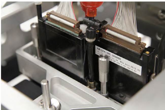
Figure 6: Example of a print head array containing over 2,000 individually addressable nozzles.
