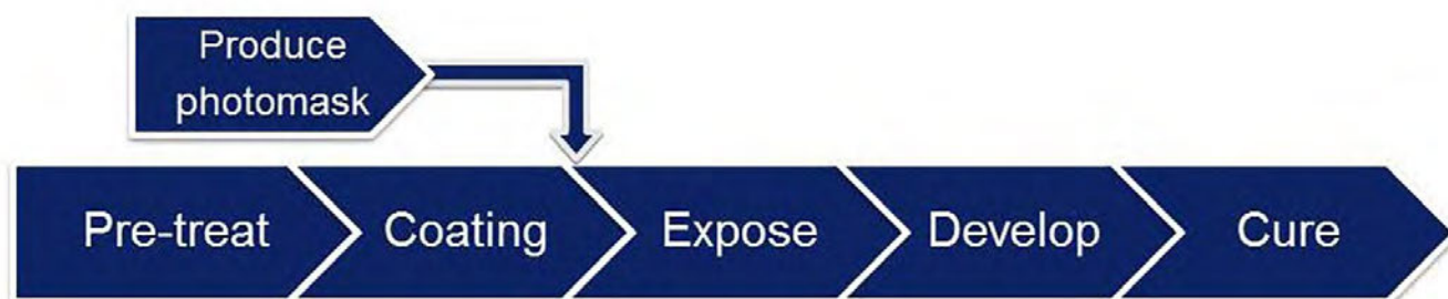
Figure 1: The process flow that is traditionally followed in PCB solder mask application.
