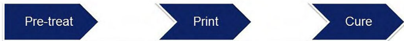
Figure 2: The process flow when using a digital inkjet printer to directly apply the patterned solder mask.
