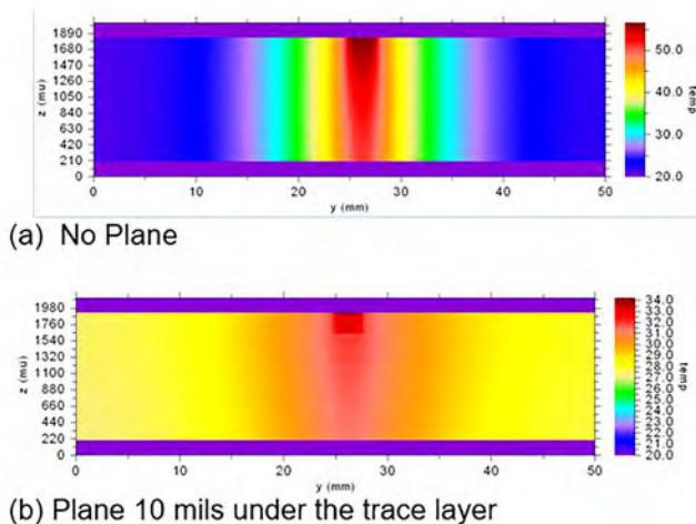
Figure 2: Thermal profiles underneath the traces and through the boards in Figure 1.
