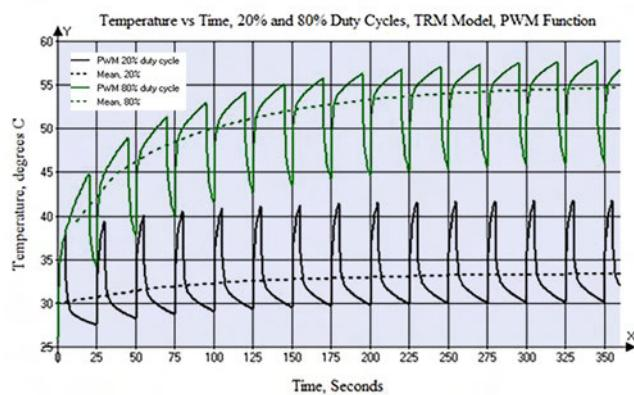
Figure 8: Temperature profiles of a trace carrying a pulsed waveform with 20% and 80% duty cycles.
