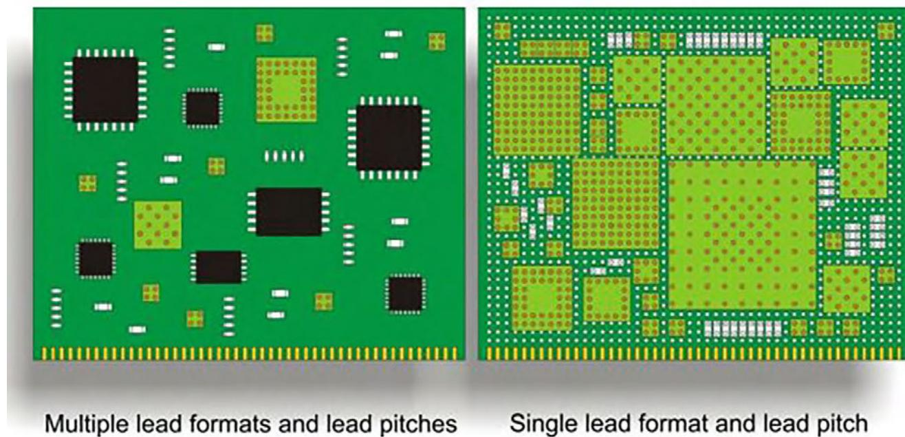
Figure 2: A variety of lead pitches shown at left, compared to the common grid on the right.
