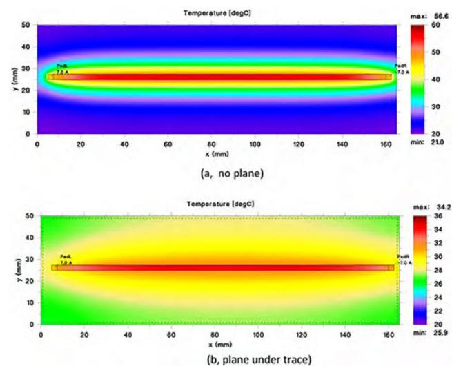
Figure 1: Thermal profile of a trace with and without an underlying plane.
