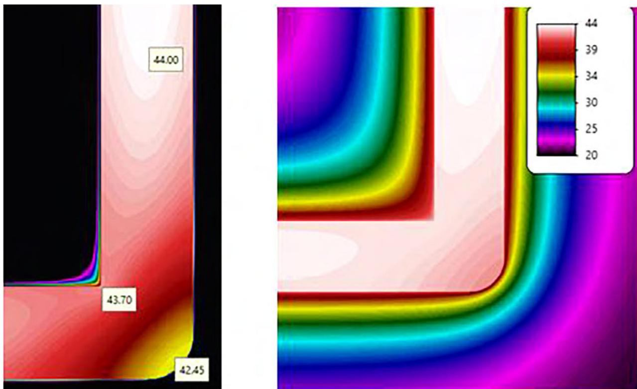
Figure 4: Thermal profiles of a right-angle corner; (a) is for a narrow temperature range, and (b) is for the full temperature range.
