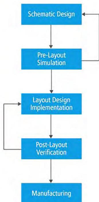
Figure 1: Advanced PCB design/analysis flow.
