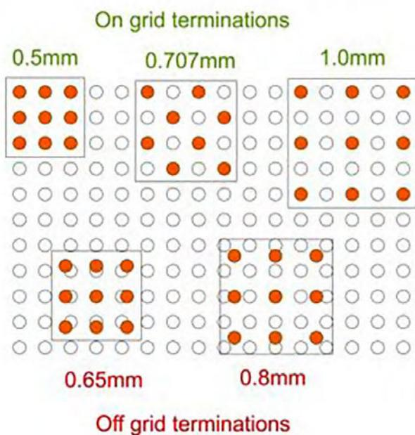
Figure 1: Basic common grid.
