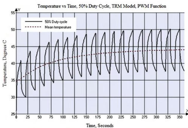
Figure 7: Temperature profile of a trace carrying a pulsed waveform with 50% duty cycle.
