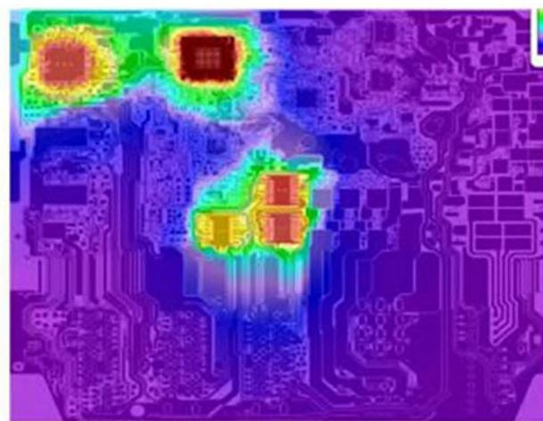
Figure 10: With TRM, a thermal profile can be generated of an entire board, including components, under load.
