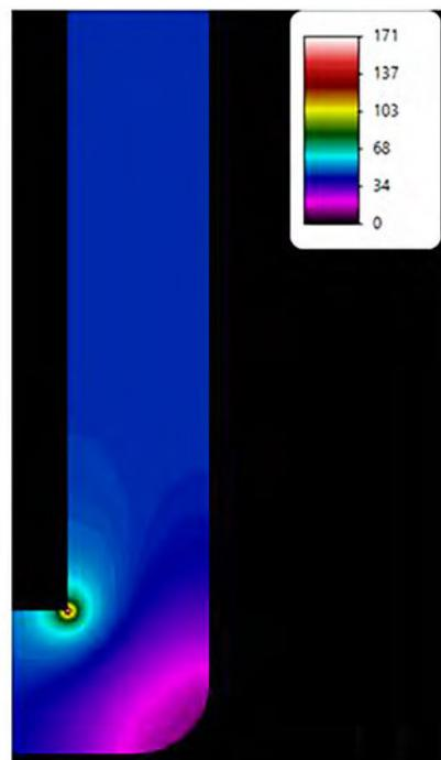
Figure 5: Current density around the right-angle corner shown in Figure 4.
