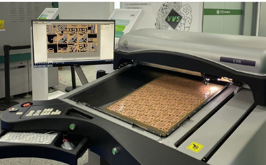
CIMS' Virtual Verification and Repair (VVR) system combines verification of AOI post-processed images with live video mode.
