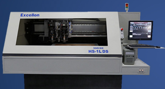
HS-1L DS Single-station, dual spindle high-speed system
