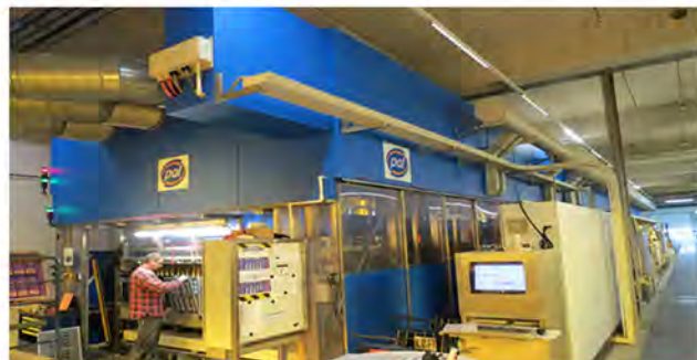
Pal Galvanic Copper-Tin Automated Electroplating Line
