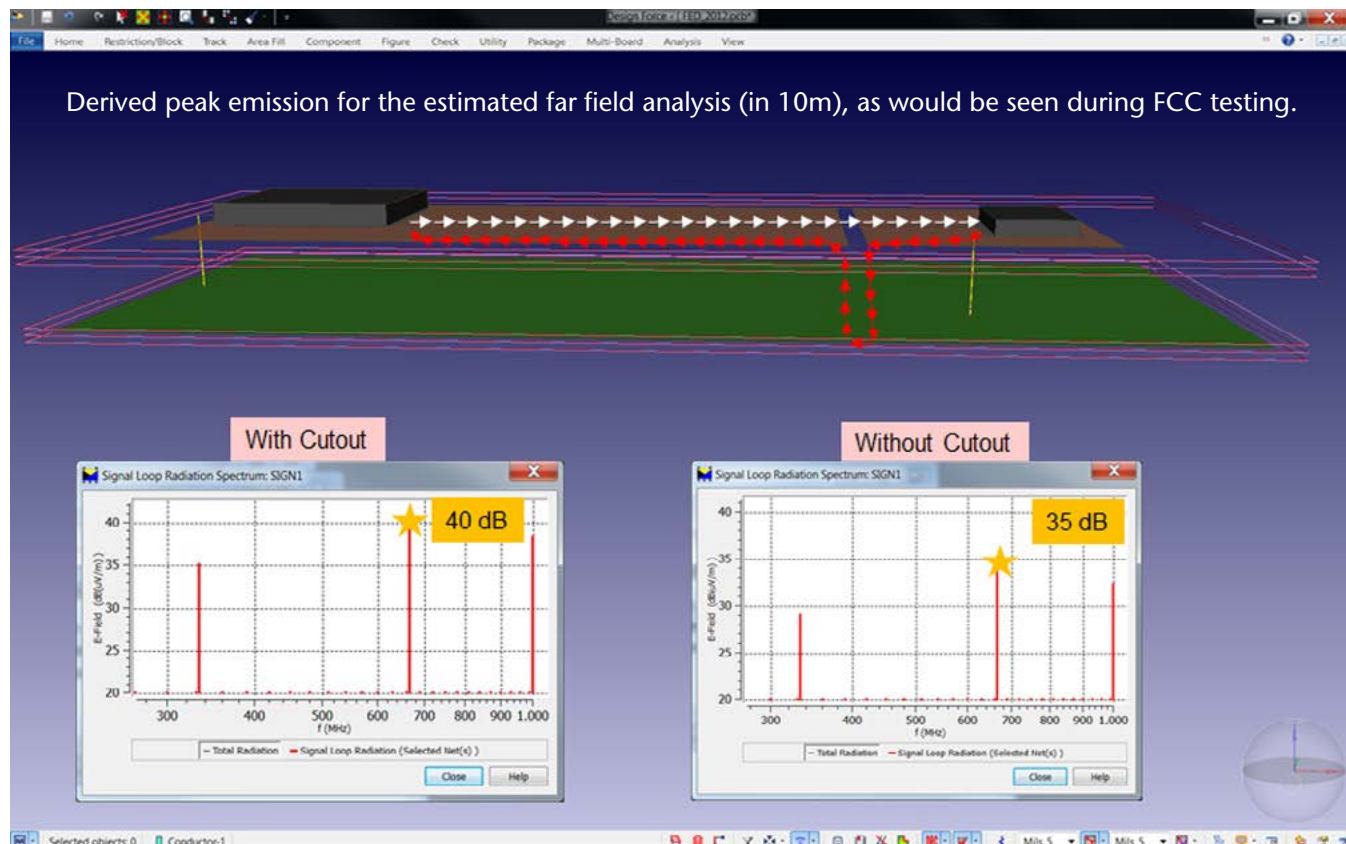
Figure 5: Estimated worst-case EMC emissions with and without reference plane cutout.
