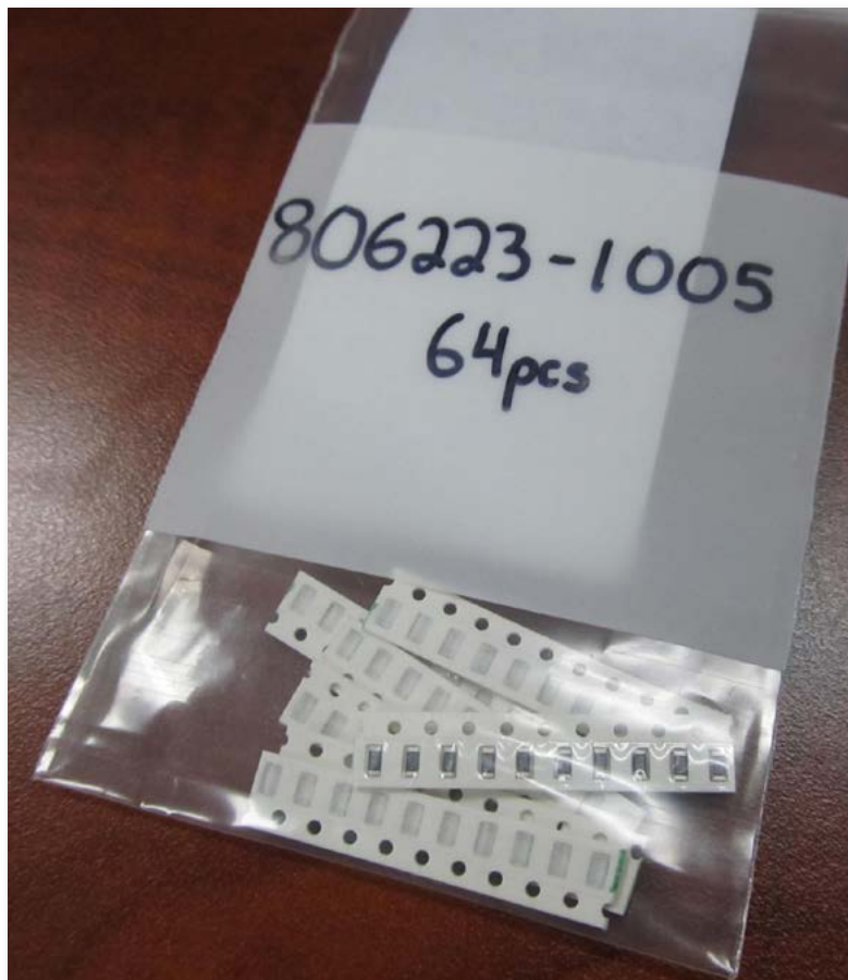
Figure 3: A proper kit would contain one contiguous tape of this component, including overage.
