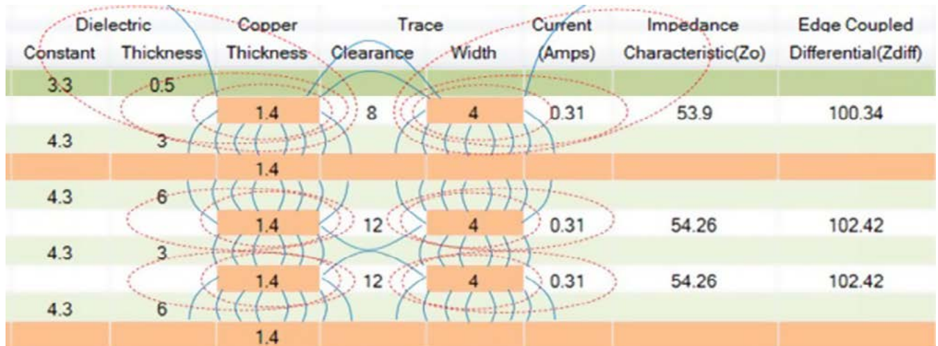
Figure 3: The electromagnetic fields as seen by the field solver in the ICD Stackup Planner.
