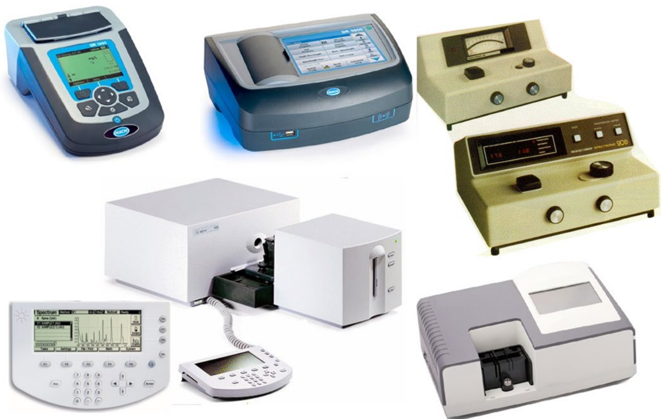
Figure 7: Six photos of common UV-VIS spectrophotometers available from laboratory supply companies and their wavelengths. Some of these have been available for the last 60 years, like the Spectronic 20.
