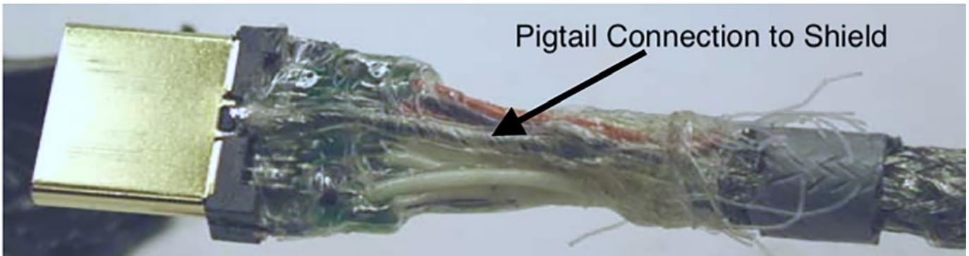
Figure 9: An example of a poor cable shield termination in an HDMI cable. (Image source: Dana Bergey)
