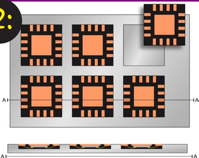
Place and bond components in cavities with copper terminations up. **Note: Vent holes can be provided in aluminum base to help planarize components.**
