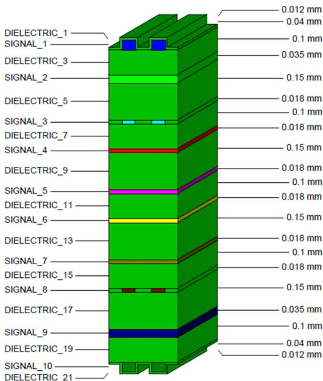
Figure 1: The control PCB featured 550 components on top and bottom side (above) and 10-layer board stackup (right).
