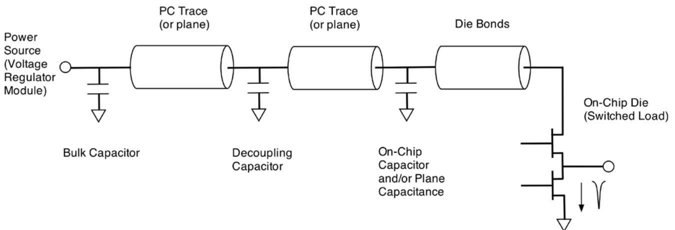
Figure 13: A typical circuit model of a power distribution network (PDN).
