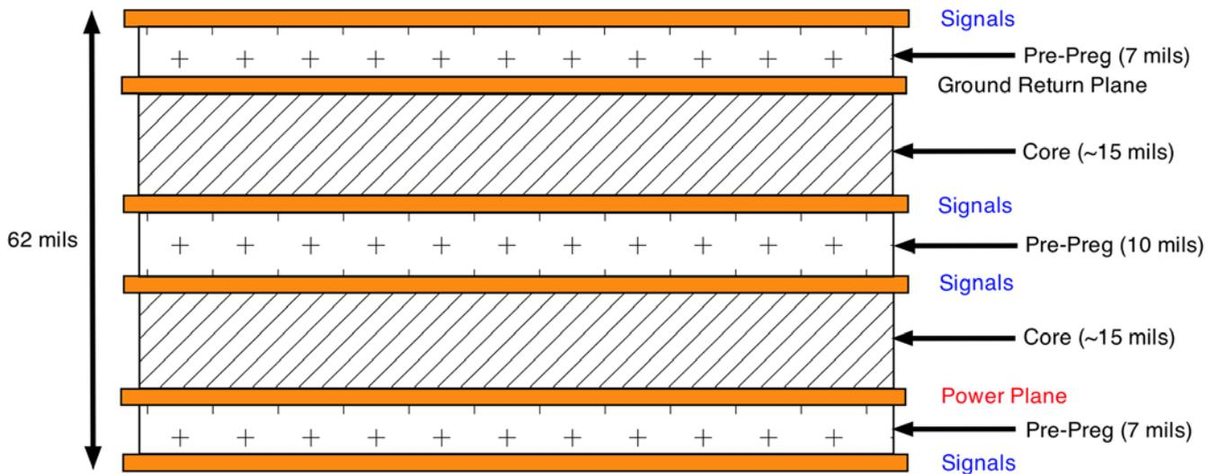
Figure 5: A six-layer board stackup with very poor EMI performance.
