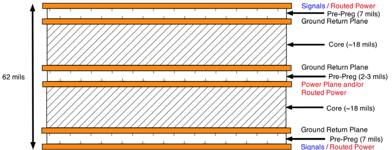
Figure 6: A six-layer board stackup with good EMI performance. Each signal layer has an adjacent return plane, and the power and power return planes are adjacent.
