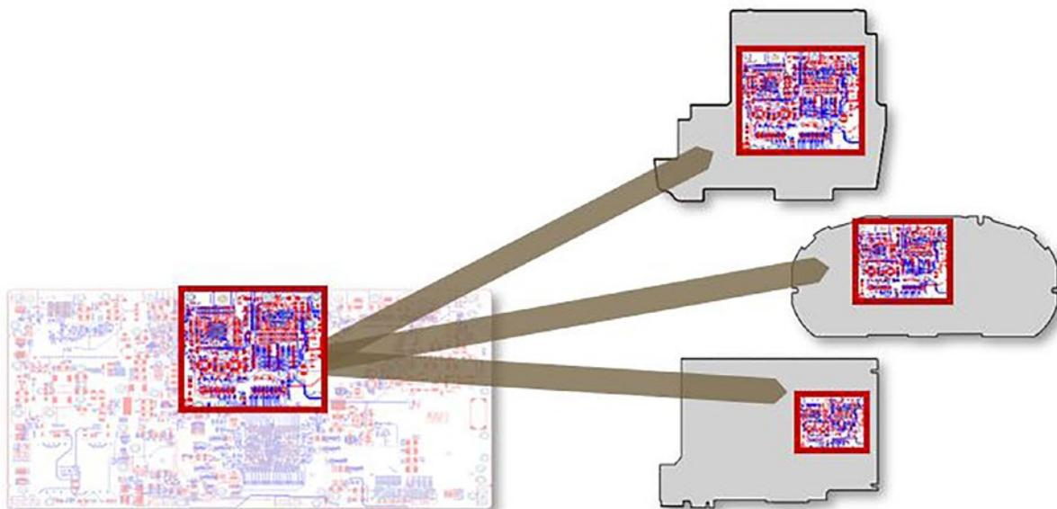
Figure 2: Example of a reuse block created from an existing known, validated, and certified CCA design.
