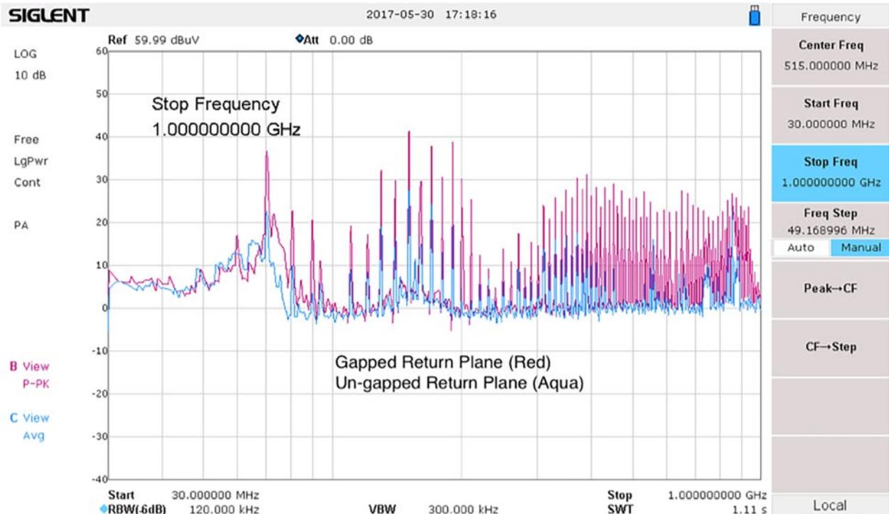
Figure 12: The resulting common mode currents on an attached wire as measured with a current probe. The trace in aqua is the un-gapped return path and the trace in red, the gapped return path. The difference is 10-15 dB higher for the gapped return path. These harmonic currents will tend to radiate and will likely cause radiated emissions failures.
