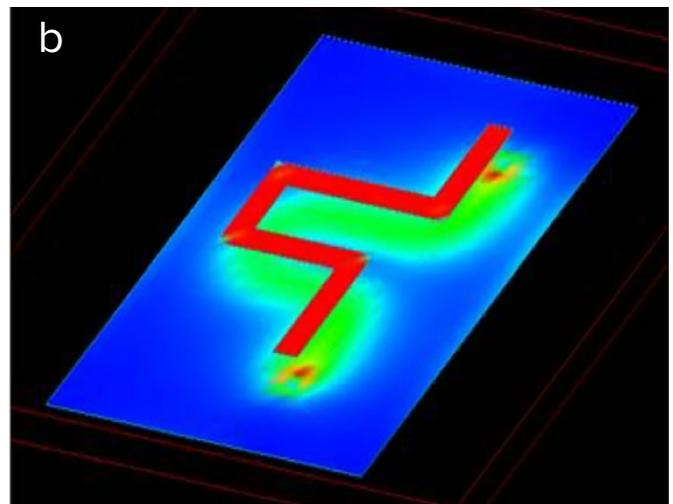
Figure 1: Simulation showing the return path (in green) at low and high frequencies. (Image source: Keysight Technologies)
