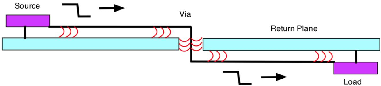
Figure 3: A signal trace passing through a single reference plane.
