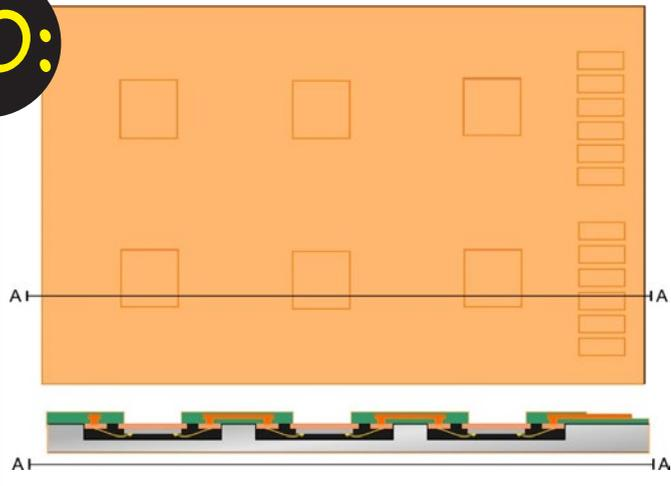
Coat assembly with electroless copper. **Note:** All surfaces are plated creating a metal encasement for the electronics.
