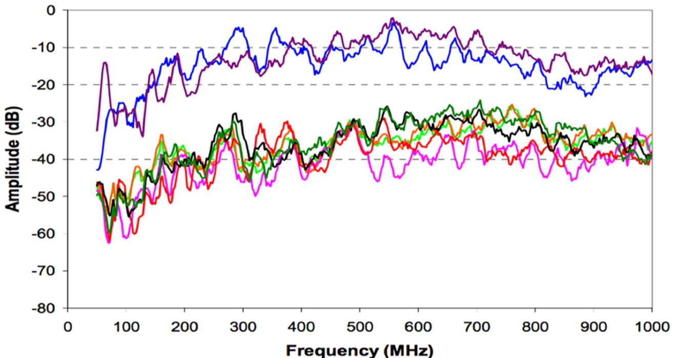
Figure 10: The results of testing eight HDMI cables from 30 to 1,000 MHz. As you can see, two of these exhibited 25 dB worse emissions across the band. (Image Source: Dana Bergey)
