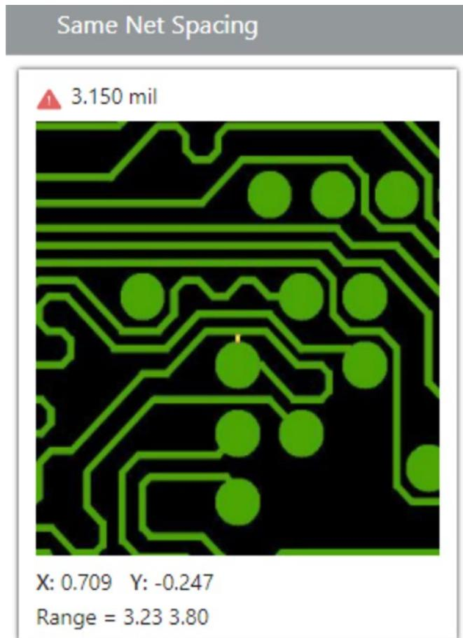
Figure 4: Constraint “same net spacing.”
