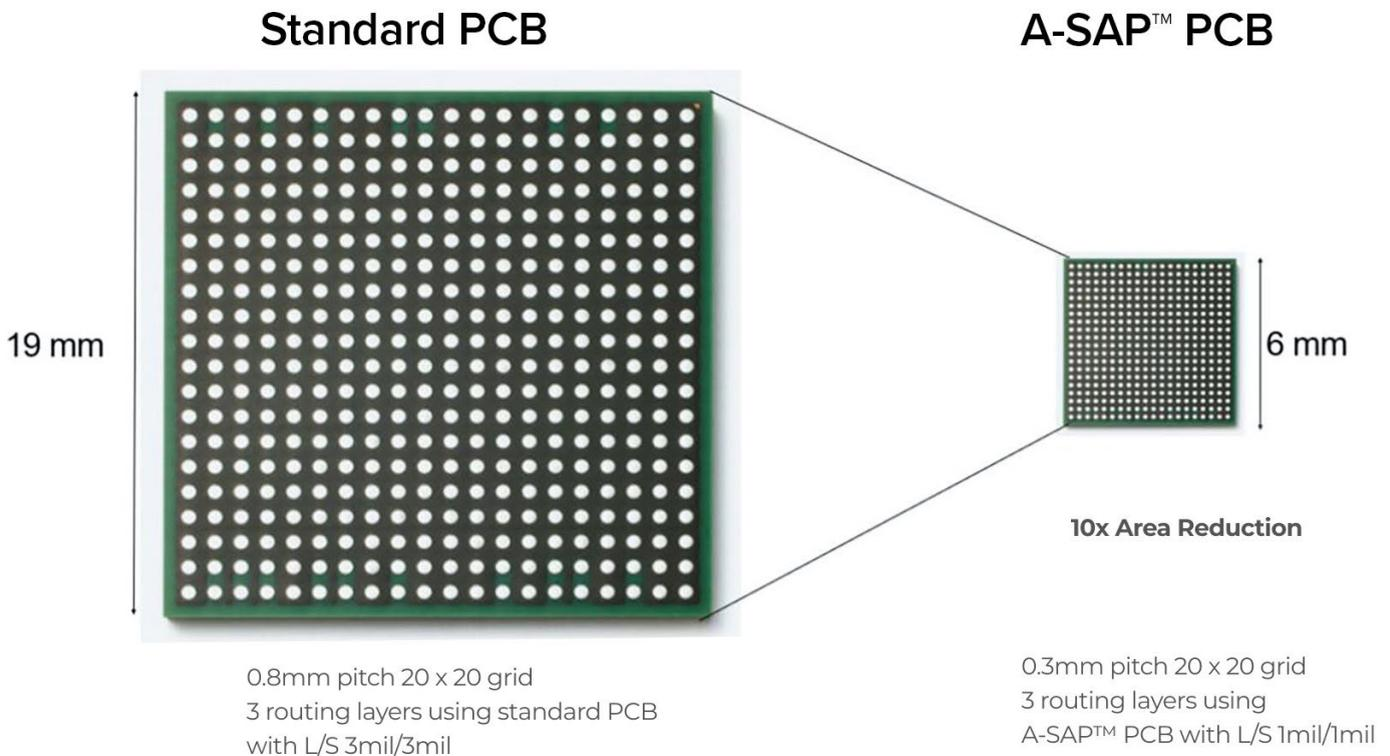
Figure 3: Many designs are being driven to require line and spaces at 50  $\mu$ m due to smaller pin spacing on components and smaller package products.
