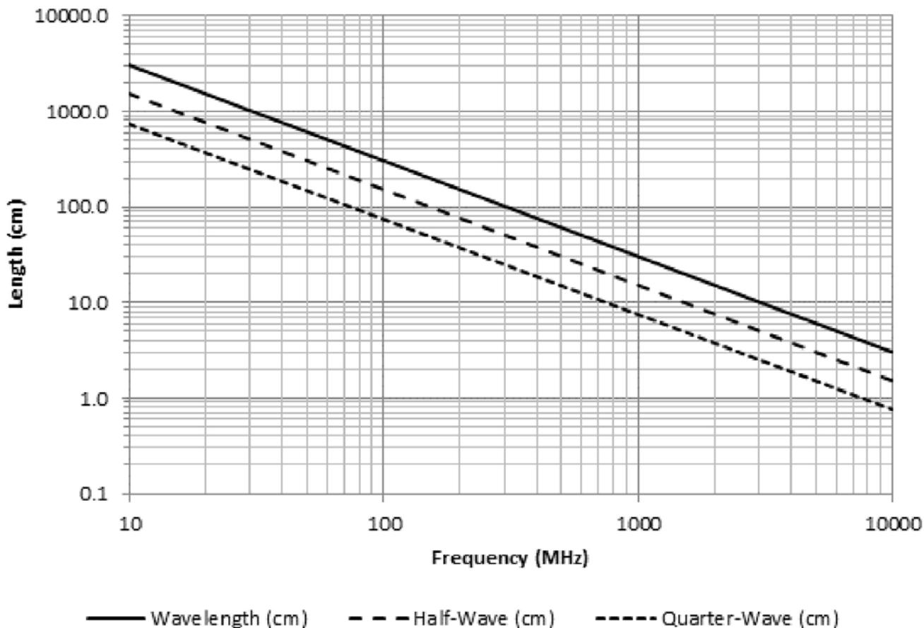
Figure 15: A handy chart for determining resonant frequency vs. cable or slot length in free space. Half-wavelength slots simulate dipole antennas and are particularly troublesome. (Image source: Patrick André)
