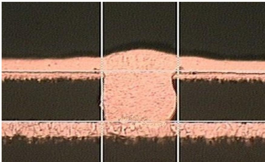
Figure 1: Copper-plated filled via showing the small dimples typically created from copper fill plating.
