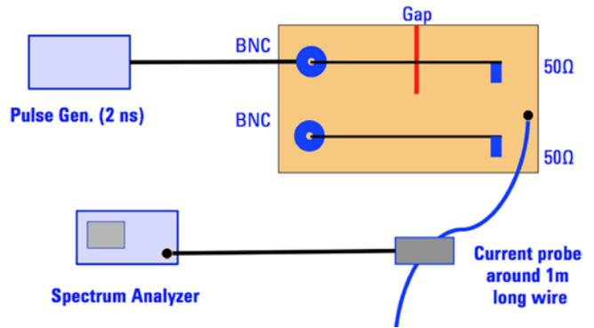
Figure 11: Shows a demonstration test board with transmission lines terminated in 50 ohms. One transmission line has a gap in the return plane and the other doesn't. A 2 ns pulse generator is connected to one of the two BNC connectors in turn and the harmonic currents in a wire clipped to the return plane are measured with a current probe.
