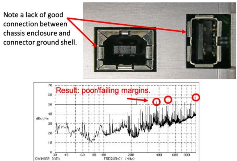
Figure 8: Result of a penetrating cable through a shielded enclosure, because of un-bonded I/O connectors to the shielded enclosure.
