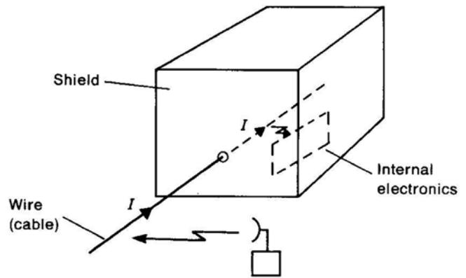
Figure 7: Penetrating the shield with a cable defeats the shield. This example shows how external energy sources can induce noise currents in I/O cables, which can potentially disrupt internal circuitry. The reverse is also true, where internal noise currents can flow out the cable and cause emissions failures. (Image Source: Henry Ott)
