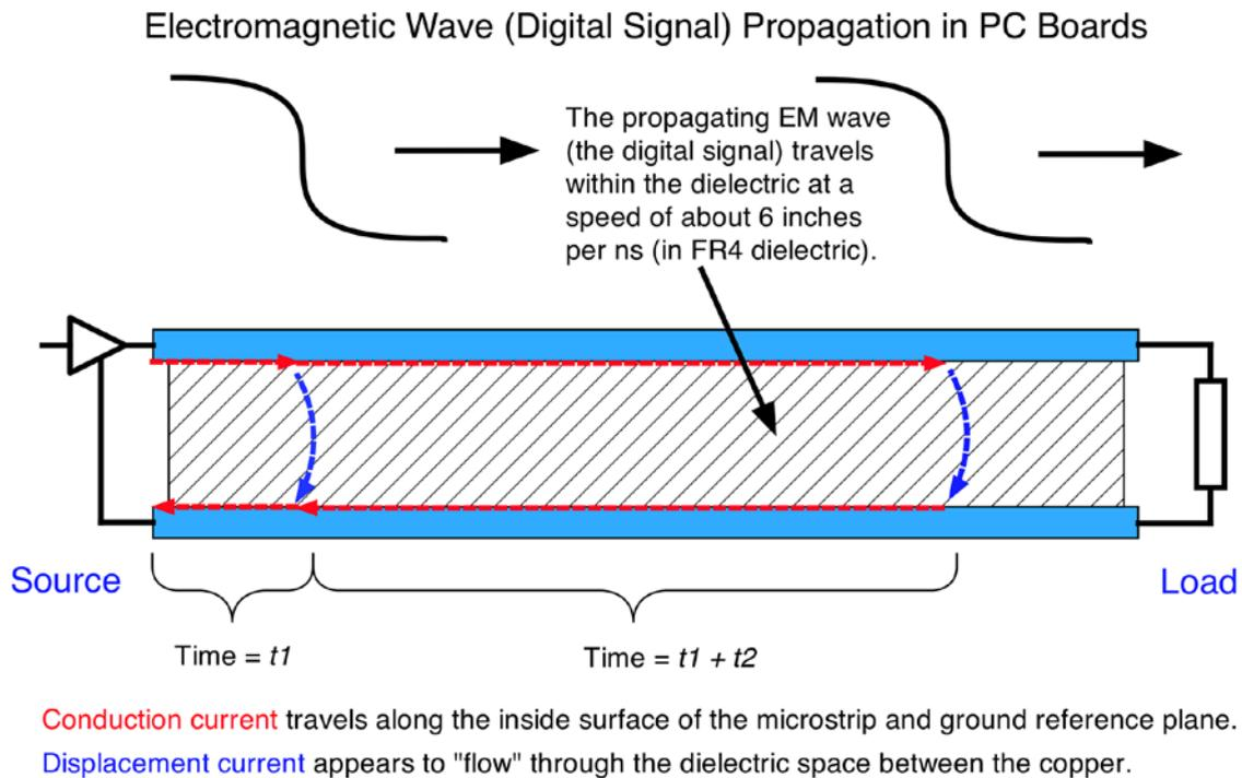
Figure 2: A digital signal propagating along a microstrip with currents shown. (Image source: Eric Bogatin)
