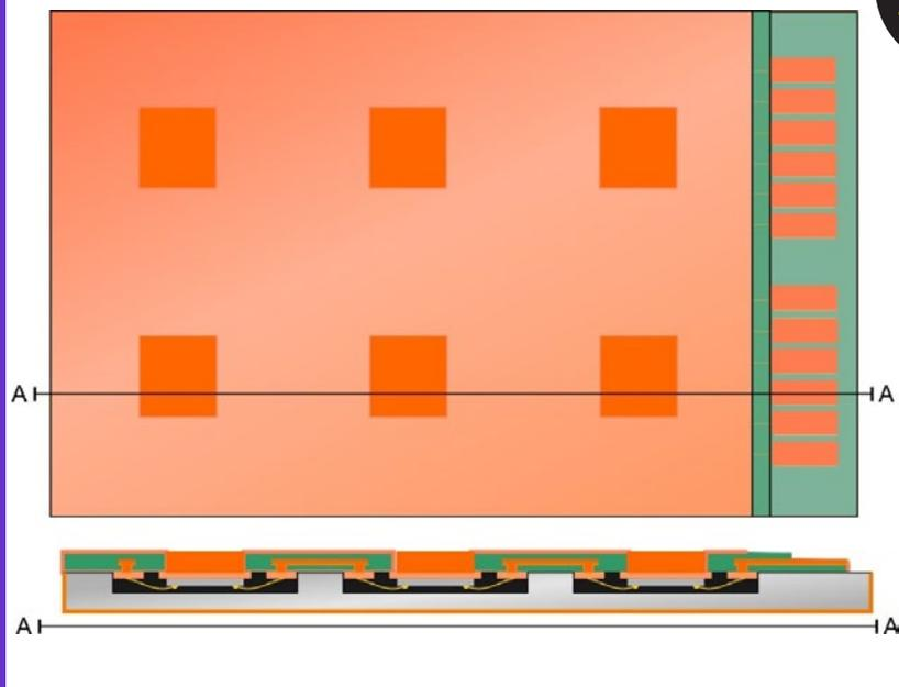
Remove tape, flash etch electroless copper, fill cavities with optional sinterable conductive paste. **Note: Metal paste brings thermal pad to surface level for better access to thermal spreader if desired.** Assembly with metal jacket is ESD and EMI immune and largely hermetic. Contacts can be gold plated.
