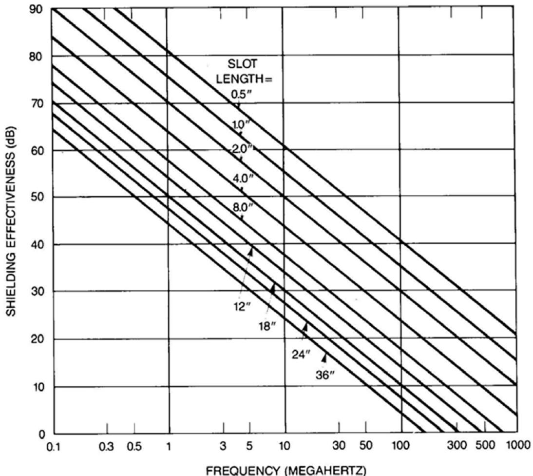
Figure 14: A chart of attenuation versus slot length. (Image source: Henry Ott)
