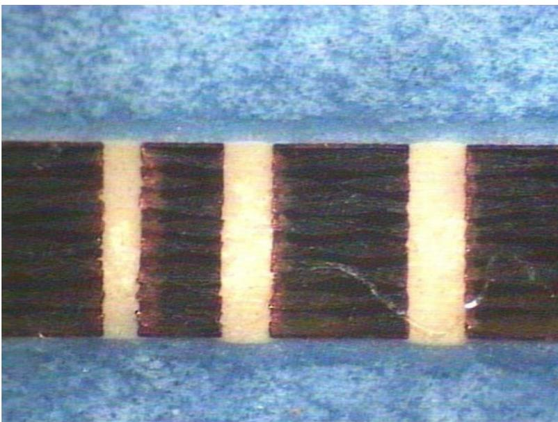
Figure 1: Example of a paste-filled through-hole.
