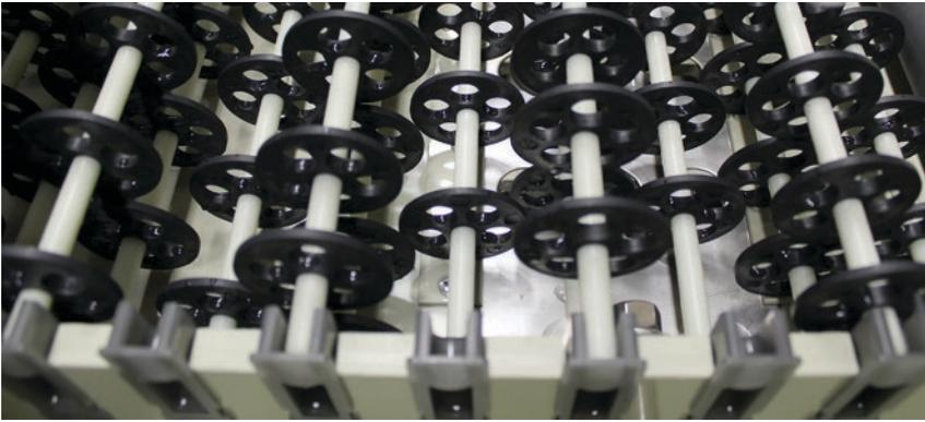
Figure 1: Standard wet processing conveyor.
