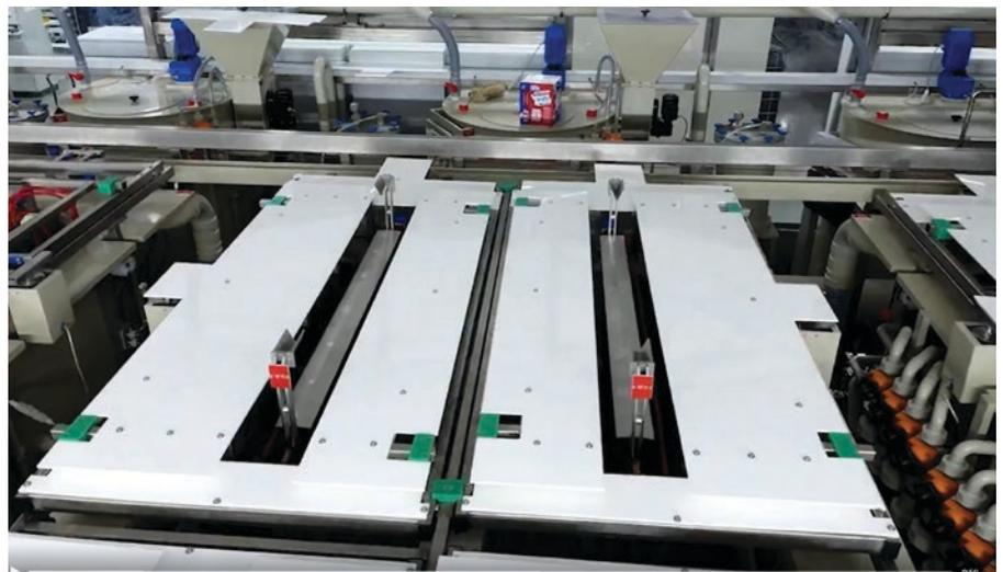
Figure 6: Process tank covers can reduce exhaust air by up to 80%. (Source: Ludy)
