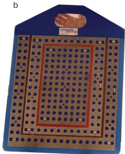
Figure 2: The use of segmented anodes, in conjunction with separate DC or pulse-plating power supplies, allows much finer control of cathode current densities and distributions. This is very important for newer copper via filling chemistries and for apparatus that employs conveyORIZED cathodes (panels).
