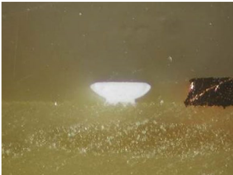
Figure 9: Example of undercut in a solder dam.
