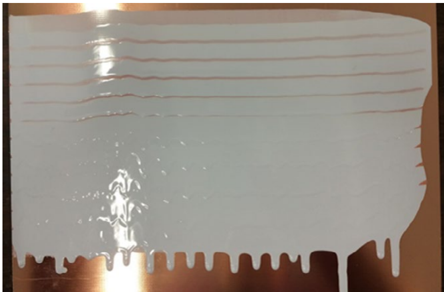
Figure 8: The panel above demonstrates sag where the drips start at the top of the panel and slump (the thicker bottom edge of the lines). The thickness ranges from 2 mil to 12 mil from top to bottom.
