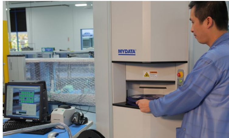
Figure 2: Humidity-controlled towers are used to store components as part of line-side stocking programs.
