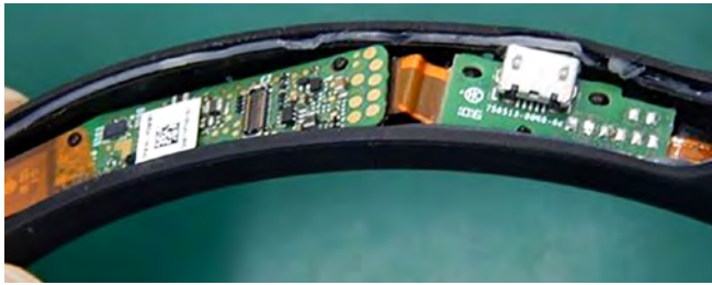
Figure 2: Bose discovered that flex is a much better fit than a rigid board for their latest electronic devices.
