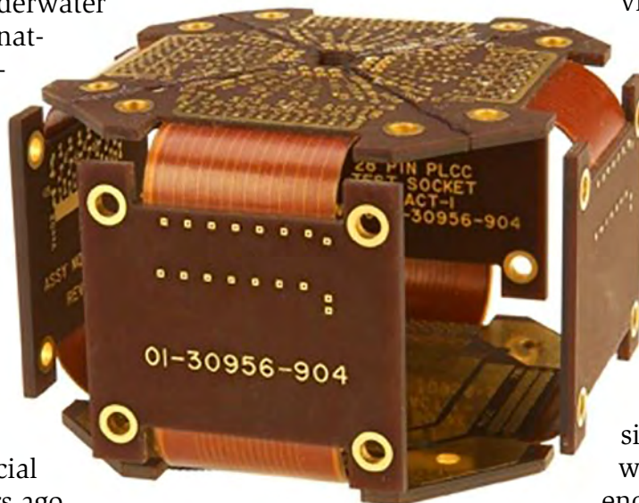
Figure 1: Rigid-flex boards allow the electronics to fit to the form of the device.
