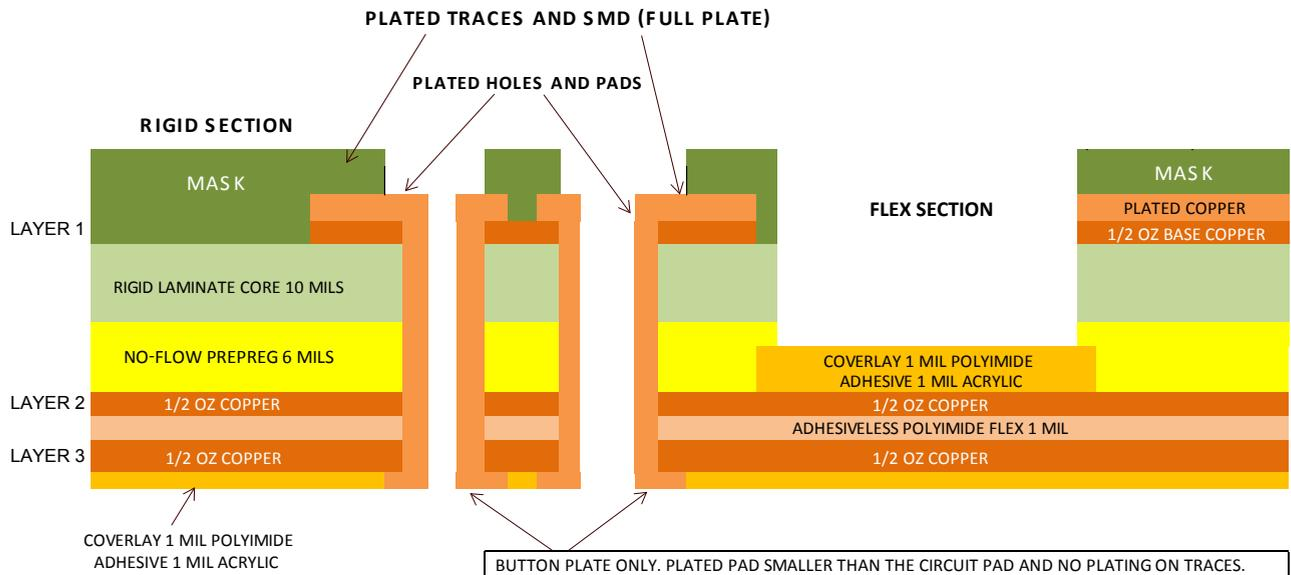
Figure 4: For extreme flexing, consider plating only the holes and pads on the flex circuit side.
