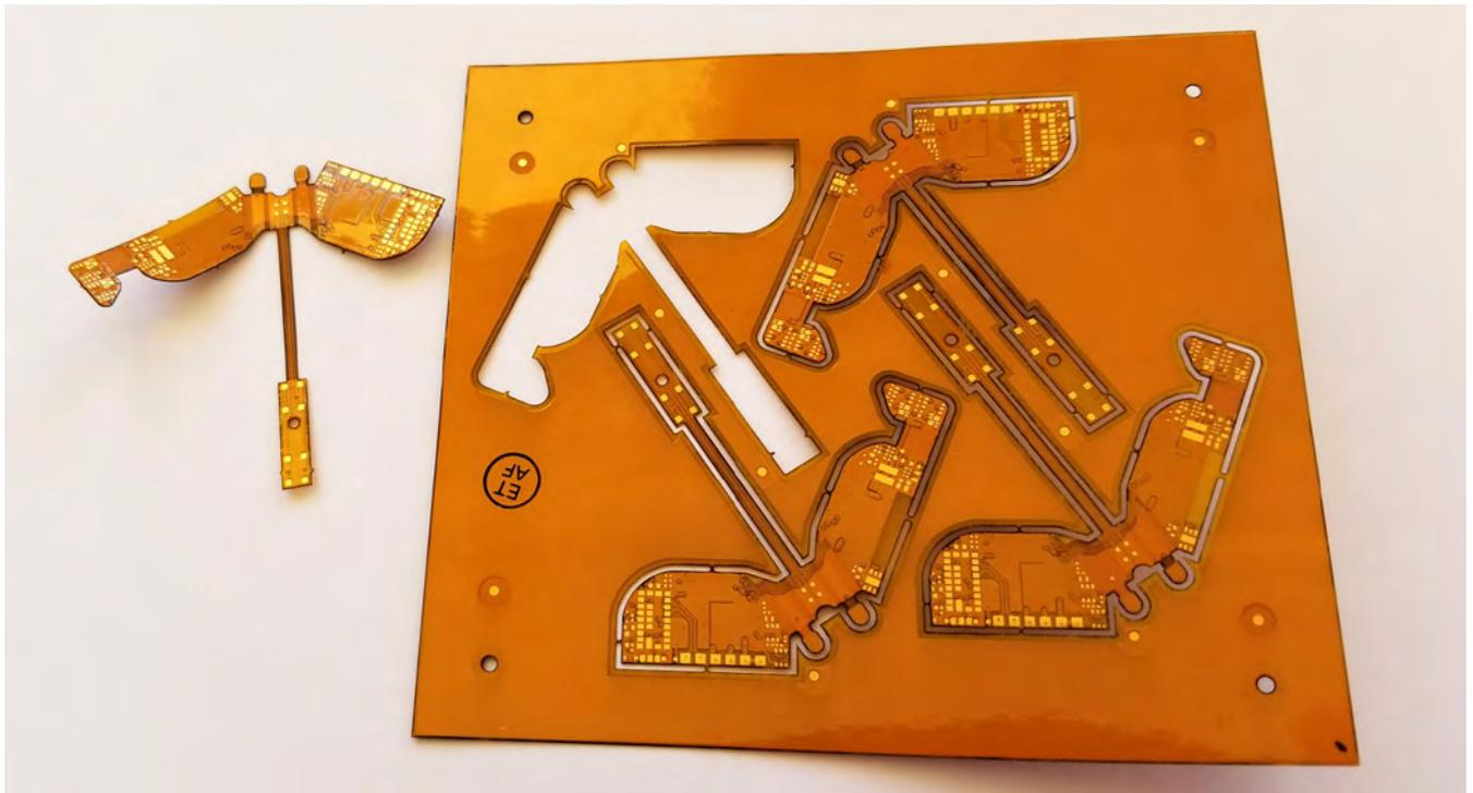
Figure 5: Odd-shaped flex circuits in panel array for ease of assembly.
