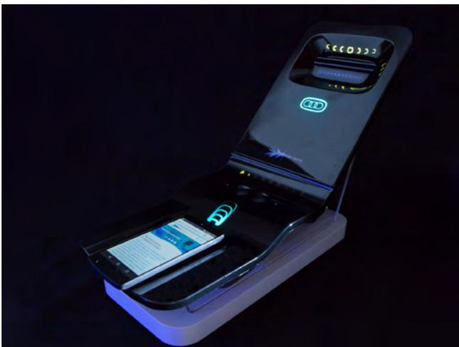
Figure 3: Thermoformed midconsole for automotive applications, including capacitive touch, OLED integration, and NFC read-out.
