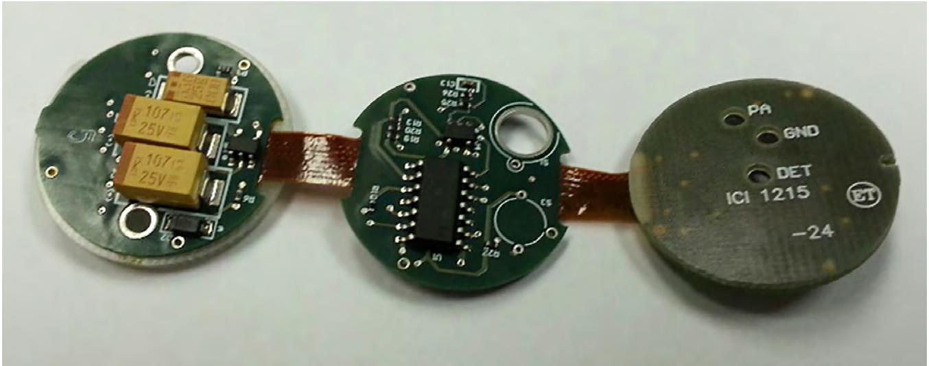
Figure 2: Rigid-flex circuit consisting of 4-layer rigid with 2-layer flex connecting each rigid section.
