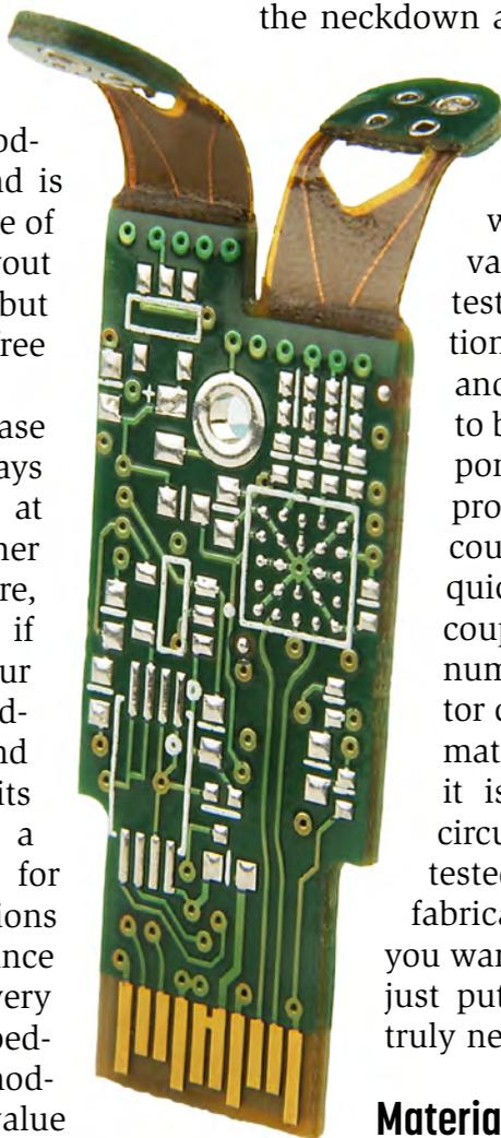
Figure 1: Six-layer rigid-flex board with controlled impedance circuitry.
