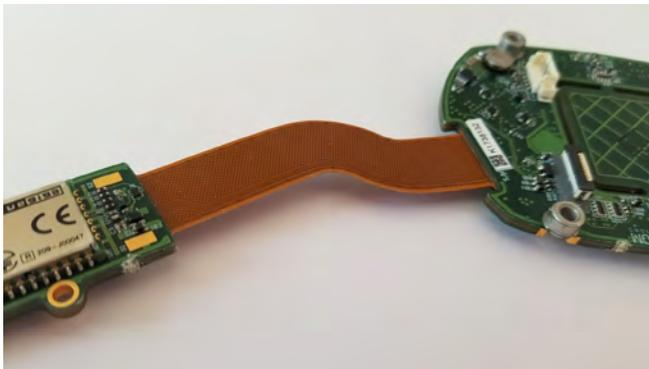
Figure 3: Rigid-flex circuit consisting of 8-layer rigid with 2-layer flex with controlled-impedance traces and filled microvias.
