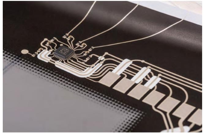
Figure 4: Circuitry printed on flat plate before thermoforming into a 3D product.
