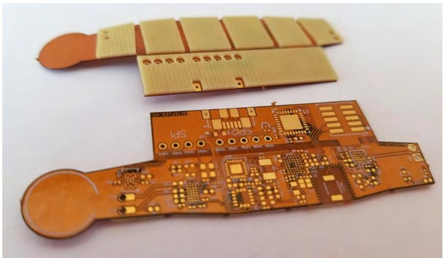
Figure 1: Four-layer flex circuit with stiffener sections on the back side to support the surface-mount components.
