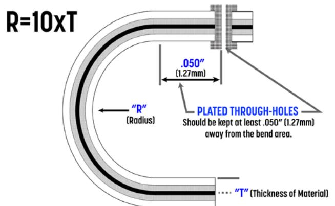
Figure 4: Flex circuit bend radius guideline.
