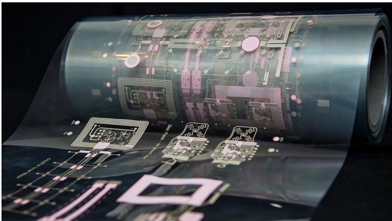
Figure 2: Roll-to-roll printed circuits on film.
