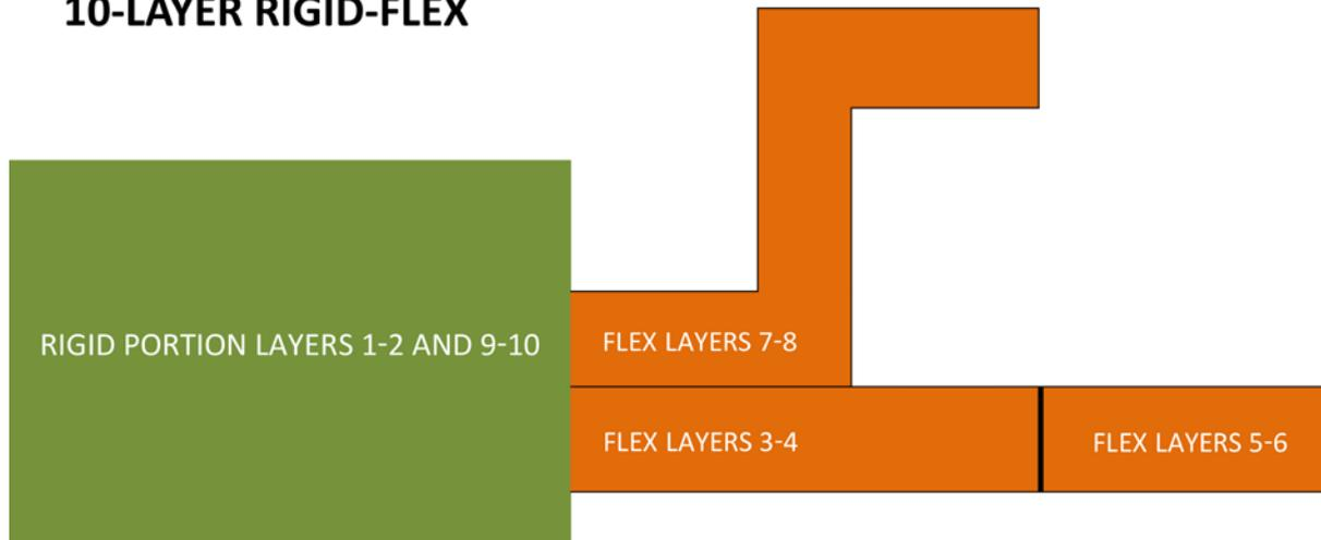
Figure 6: 10-layer rigid-flex with multiple layer separation and discrete routes.
