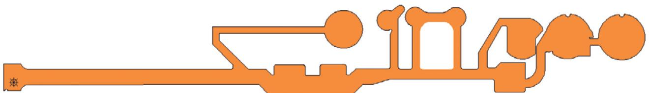
Figure 5: Flex with multiple discrete breakout section.
