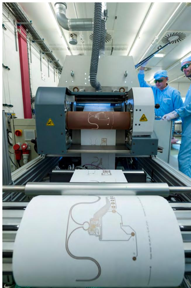
Figure 1: Roll-to-roll printing of circuit on films at a maximum speed of 60 m/min.
