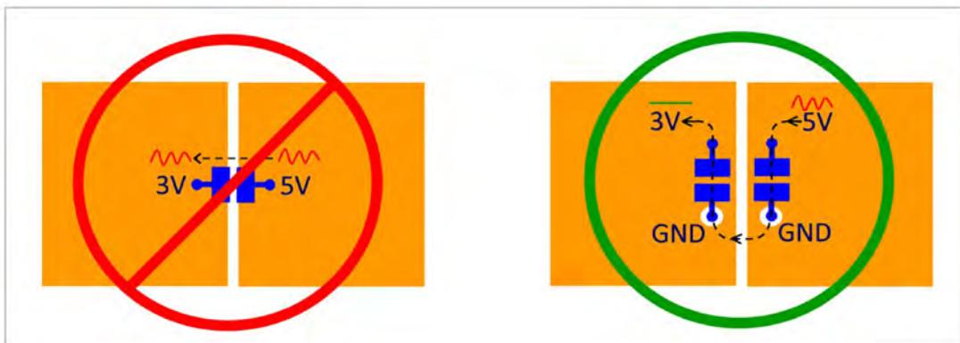
Figure 4: Eliminating the transfer of noise in the return path of split power planes (right).
