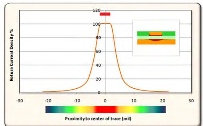
Figure 2: Microstrip return current density.
