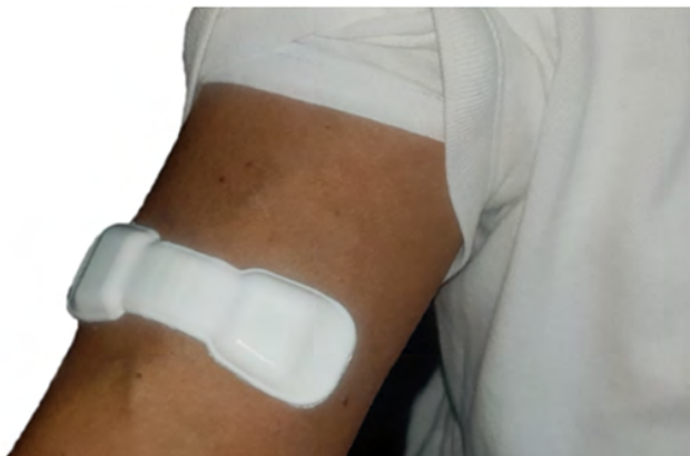
Figure 3: Molded GraftWorx SmartPatch. Extremely flexible regions allow for conformal application on the body. Silicone molding and special gasketing enable the patch to meet IP-64 (splashing/shower) requirements.
