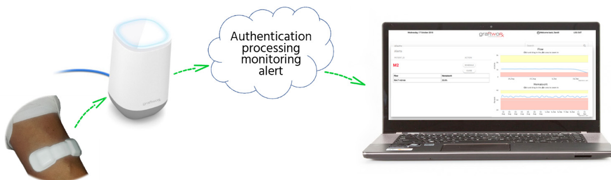
Figure 1: The GraftWorx end-to-end data path. Results from patient monitoring are transmitted via a semi-custom Bluetooth link to our B2H data bridge. Data is transmitted over a cellular IoT network to the Cloud where, after authentication, data is processed and alerts generated. Data and alerts are available to clinicians as part of their standard clinical workflow.
