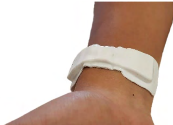
Figure 3: Molded GraftWorx SmartPatch. Extremely flexible regions allow for conformal application on the body. Silicone molding and special gasketing enable the patch to meet IP-64 (splashing/shower) requirements.
