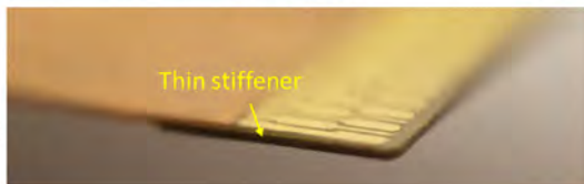
Figure 6: The design and construction of dual-row ZIF connectors makes them vulnerable to cracking.
