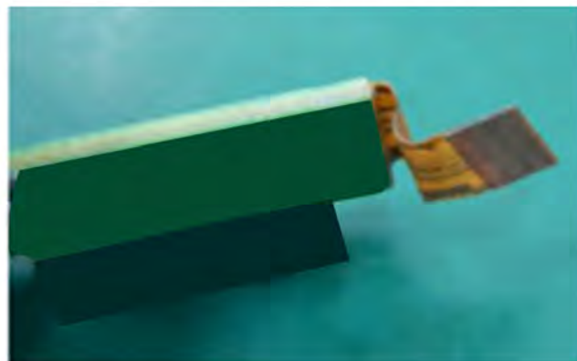
Figure 8: A pre-bend fixture was developed and implemented to ensure predictable and repeatable bend of the flex tail with the ZIF fingers (L), and the rigid-flex circuit after pre-bend (R).
