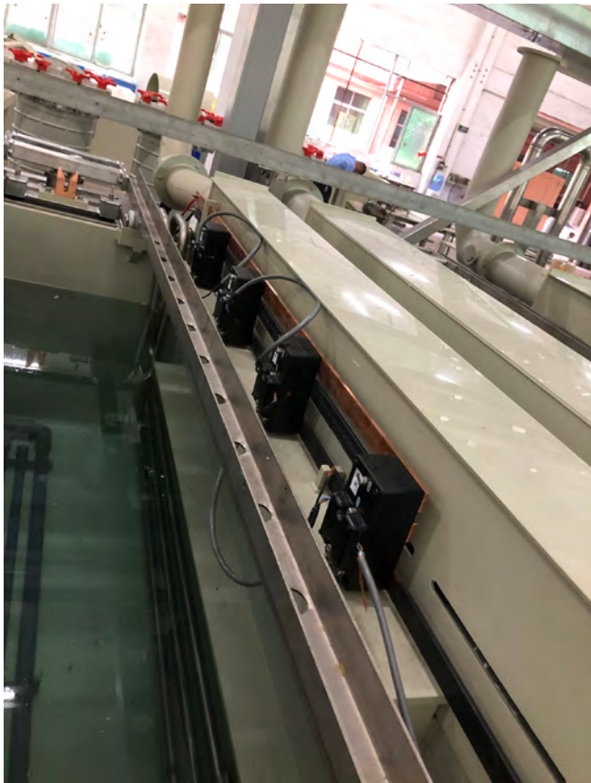
Figure 2: Multiple rectifiers anode bar.
