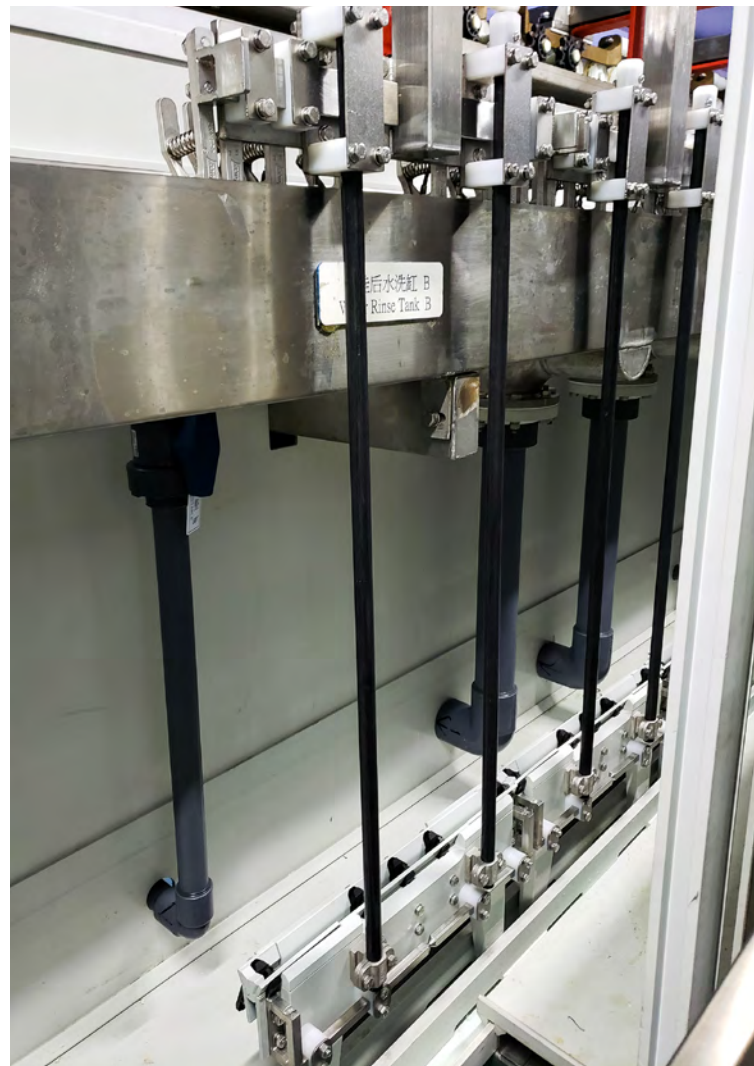
Figure 3: Top and bottom VCP clamps.
