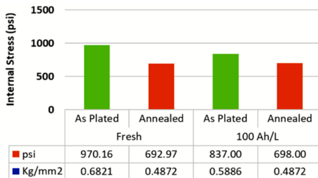
Figure 9: Internal stress of the copper deposit plated using Process I, both as plated and annealed data for fresh and aged baths.
