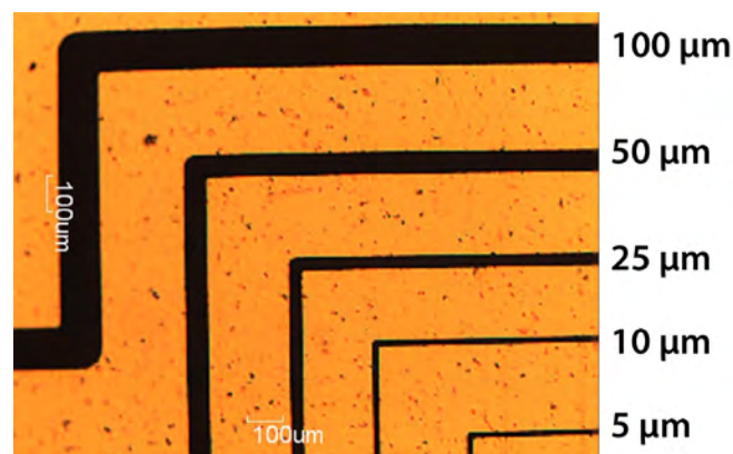
Figure 8: Test pattern formation with a full additive process.
