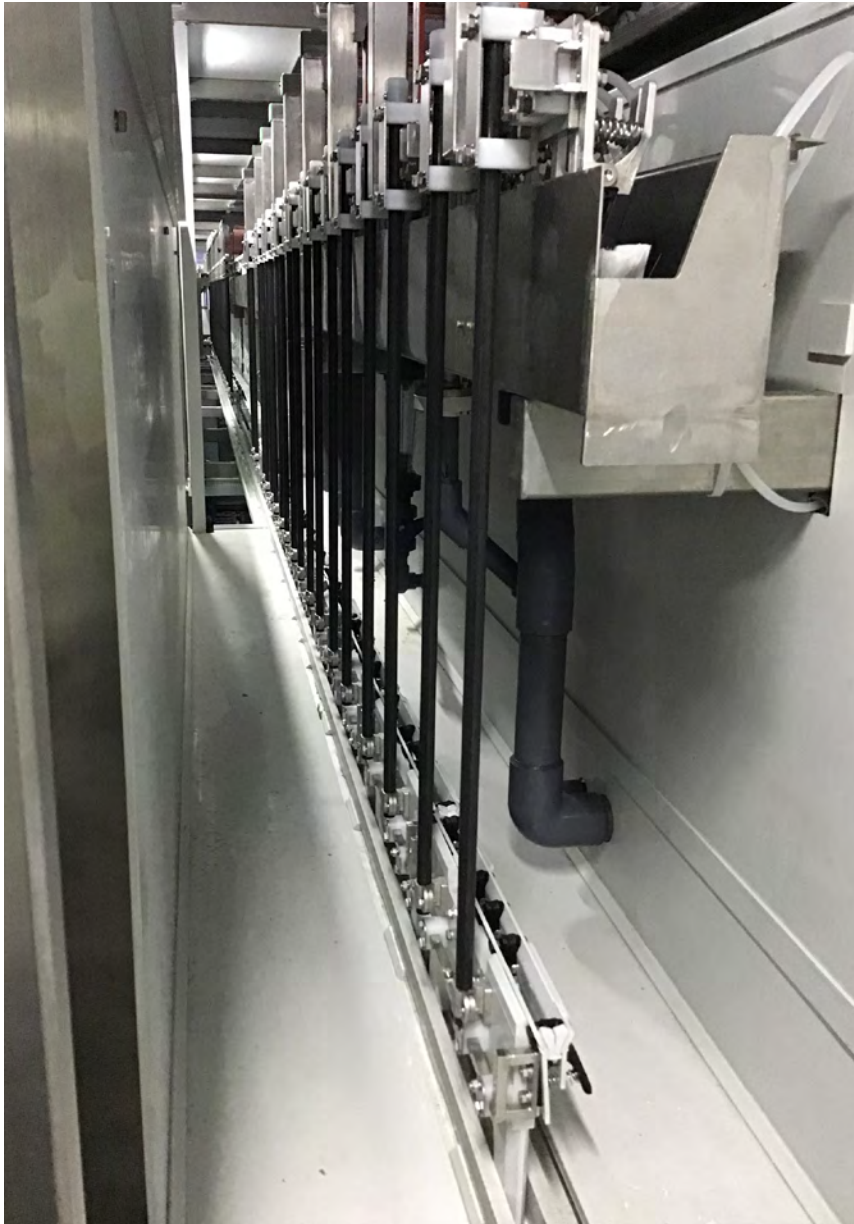
Figure 4: Top and bottom VCP clamps.
