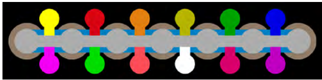
Figure 13: Mechanical symbol placed in the design, BGA pin drive connection via net name.
