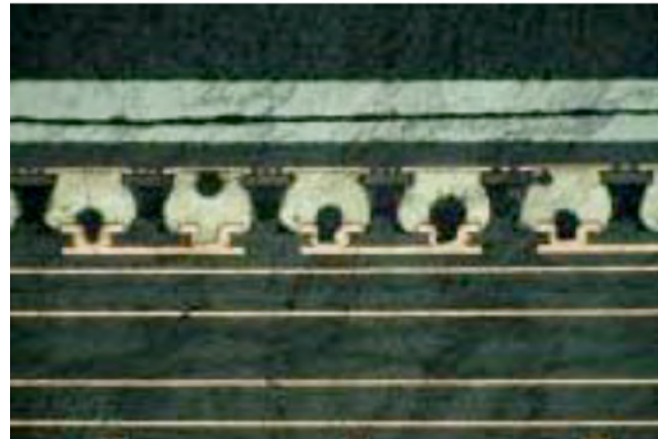
Figure 2: Component mounted on unfilled vias (note the air pockets).
