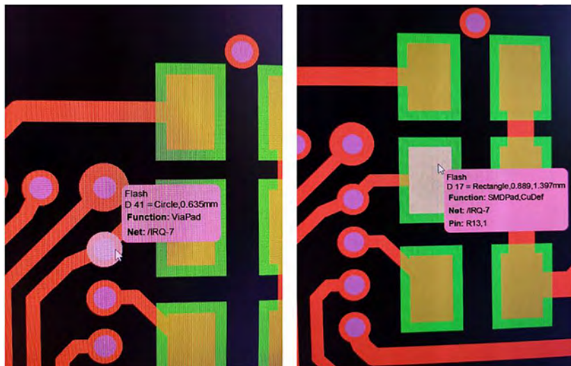
Figure 1: Output from a popular CAD system illustrates that Gerber X2 fully identifies pad types, sizes, nets, and pins.
