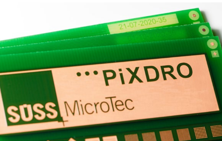
Figure 3: Example of serialization of panels in clear sight, hidden or absent.
