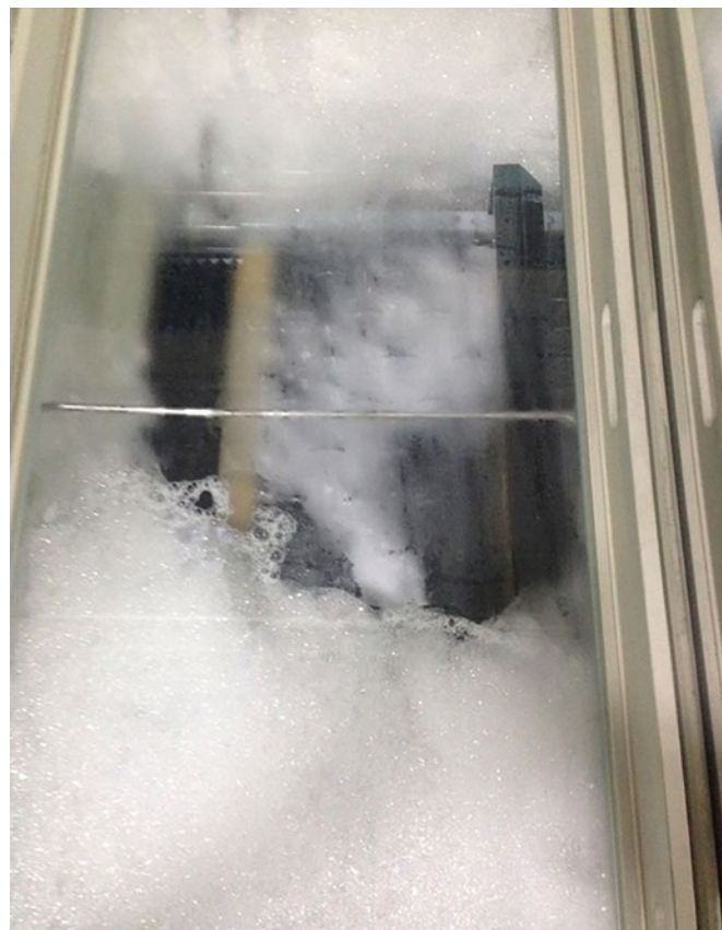
Figure 3: Poor rinsing leading to cleaner drag-in to another key process tank: Significant foam from residual cleaner drag-in.
