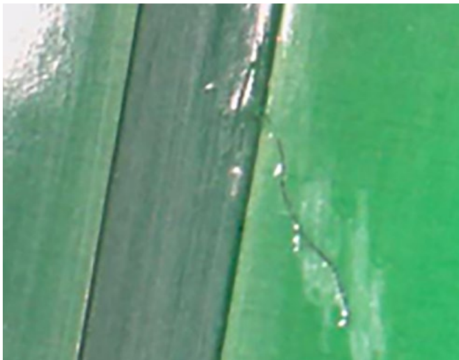
Figure 2: An unwanted particle in solder mask not violating general rules but still not allowed by the workmanship requirement.
