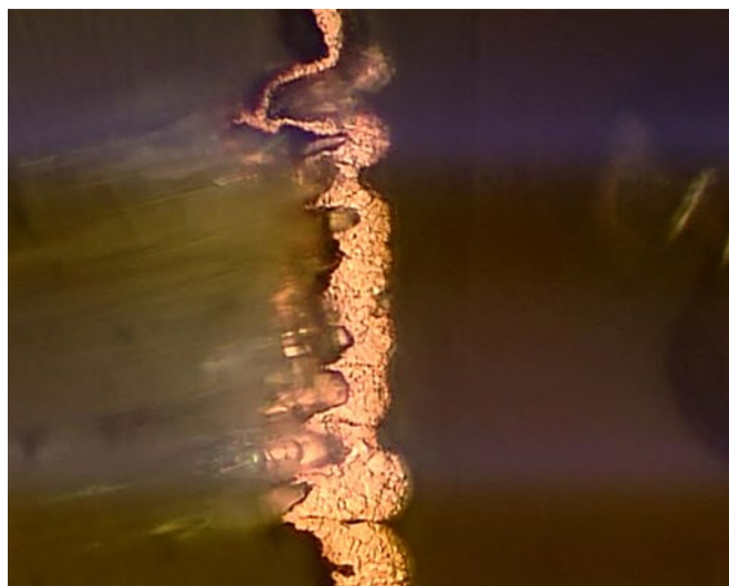
Figure 1: Extreme rough hole wall due to poor drilling practices.
