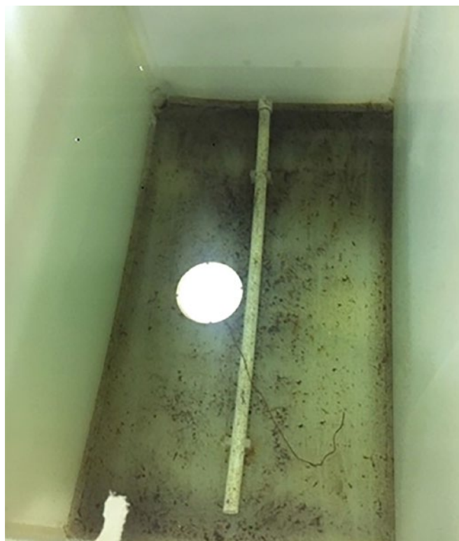
Figure 6: Sediment remaining in a process tank that used no filtration.
