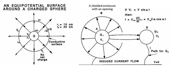
Figure 2: Remember: If you have one conductor, such as a sphere, with no hole in it (2a), any EM field contained inside the sphere cannot escape. If there is only one conductor and a space (2b), the field will not be contained. (Images courtesy of Ralph Morrison, consultant)
