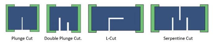
Figure 2: Laser trim variations for thick film resistor elements. (Trim examples courtesy of PPI Systems)
