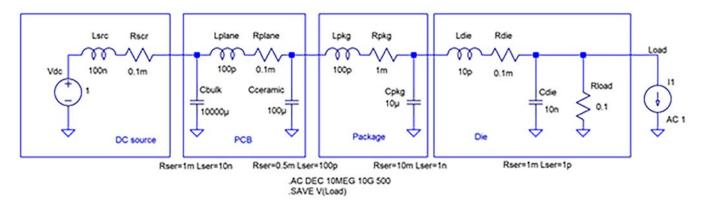
Figure 2: LTSPICE schematics of a simple point-of-load PDN.
