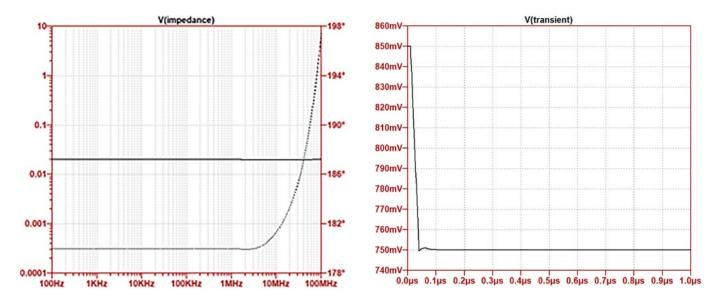
Figure 4: Impedance profile (on the left) and transient response (on the right) of the circuit in Figure 3.
