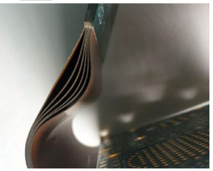
Figure 3: Completed PCB flex belts separated.
