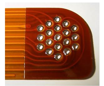
Figure 1: Reinforced flex for soldering to military connector.
