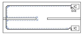
Figure 1: If the return plane is split, the field must fill the space between the signal trace and the ground copper. (Image courtesy of Rick Hartley, consultant)
