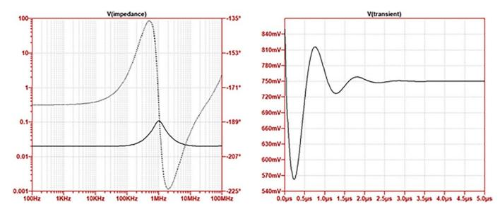
Figure 5: Impedance profile (on the left) and transient response (on the right) of the circuit in Figure 2 when we change the series inductance from 1 nH to 10 nH.
