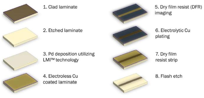
Figure 1: A-SAP<sup>™</sup> process flow diagram.
