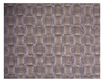
Figure 6: Flattened glass cloth/epoxy resin weave. (Courtesy of Ventec International Group)
