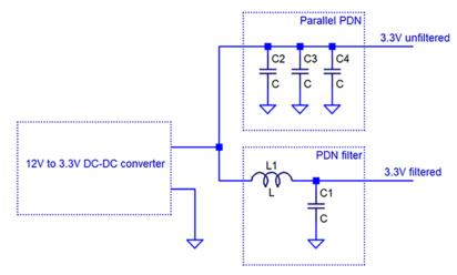
Figure 1: Block schematics of a system PDN illustrating the definitions of parallel PDN and PDN filter.
