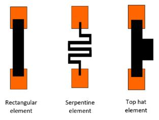
Figure 1: Thick film resistor pattern variations.
