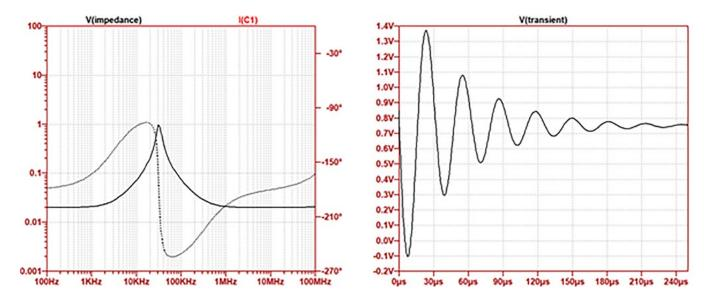
Figure 7: Impedance profile (on the left) and transient response (on the right) of the circuit in Figure 6.
