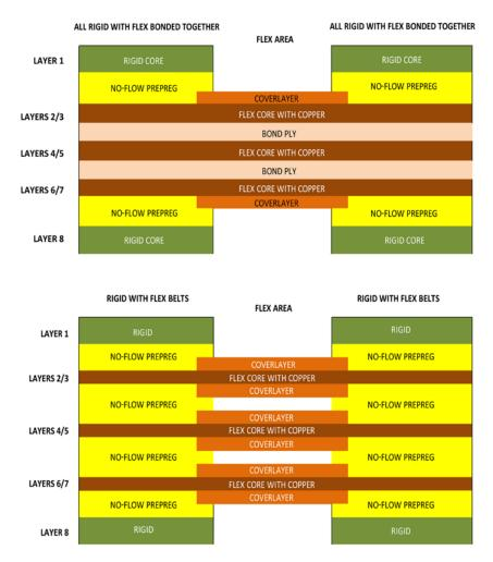
Figure 2: Bonded vs. unbonded flex areas.
