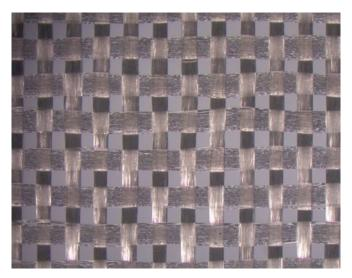
Figure 5: Traditional glass cloth/epoxy resin weave. (Courtesy of Ventec International Group)
