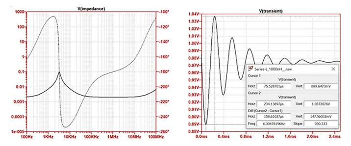
Figure 9: Impedance profile (left) and transient response (right) after we decrease AC losses by tenfold.
