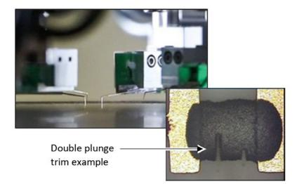
Figure 3: Laser trim system equipped with flying probe contactors. (Source: PPI Systems)
