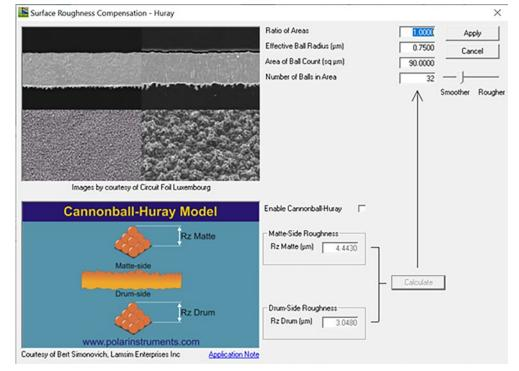
Figure 7: Modeling roughness with SEM or Cannonball model.
