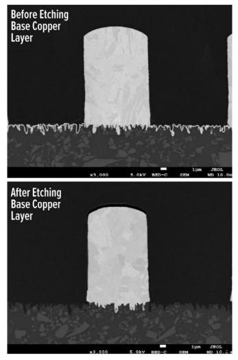
Figure 2: Before and after etching the base copper layer. (Images courtesy of MEC Corporation)
