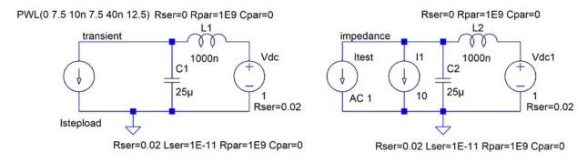
Figure 6: The circuit of Figure 3 with 1000 nH inductance and 25 mF capacitance.
