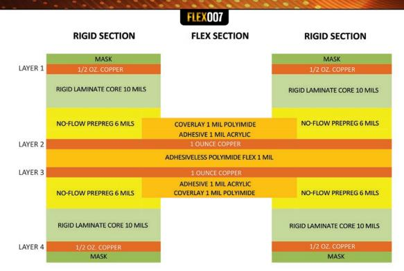
Figure 1: Example of four-layer flex construction.
