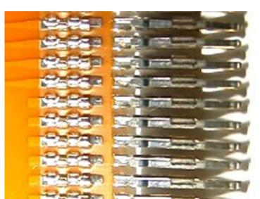
Figure 2: Pierce type connector for flex to rigid header.
