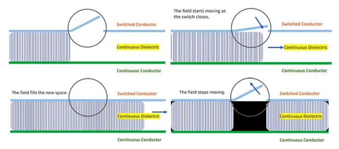
Figure 3: Images depicting the movement of an EM field as a switch closes. There are only three things that you can do with EM fields: Store them, move them, or convert them into kinetic energy.
