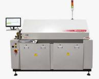
4-Zone inline reflow oven with predictive profiling
