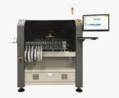
Pick & place with 160 feeder ports and 6,400 CPH placement
