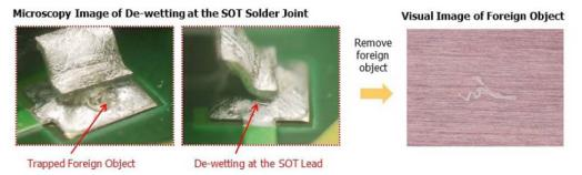
Figure 17: Microscopy image of de-wetting at the SOT solder joint and visual image of foreign object debris.
