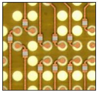
Figure 3: Subsurface conductor layer with formed thin-film resistors. (Image source: Ohmega Technologies, Inc.)
