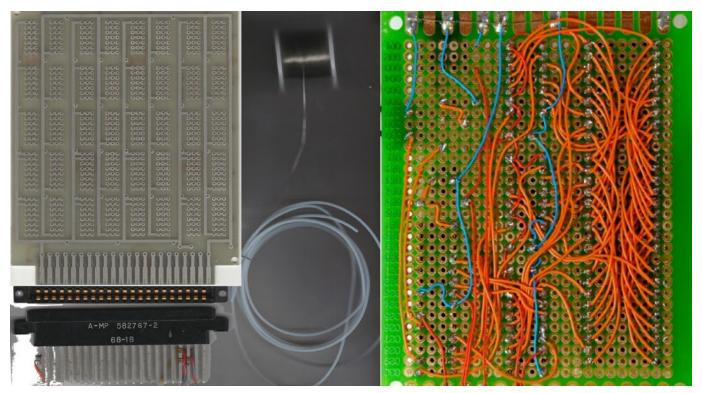
Figure 5: Bare tin-lead breadboards were manually wired with tin-coated copper wire and insulators for all the custom electronics, even by the electrical engineering and computer science departments.
