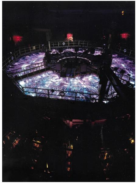
Particle Beam Fusion Accelerator firing in the 1980s. (Source: Sandia National Laboratory)
