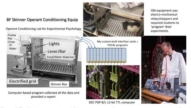
Figure 4: The food sensor-equipped Skinner boxes used for experiments on rats were interfaced via custom PCBs to the new DEC PDP 8/L minicomputer, replacing the old electro-mechanical steppers and relays that were unreliable and difficult for students to program.
