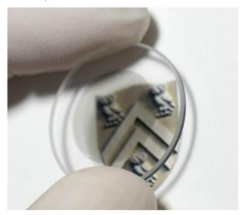
This rotation doesn't mean the films are spinning. It does mean that polarized light from a laser or other source can now be manipulated in ways that were previously out of reach, making it completely visible or completely opaque with a device that's extremely thin.
