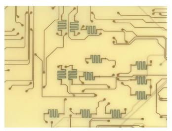
Figure 4: Serpentine-configured thin-film resistor examples. (Image source: Ohmega Technologies, Inc.)
