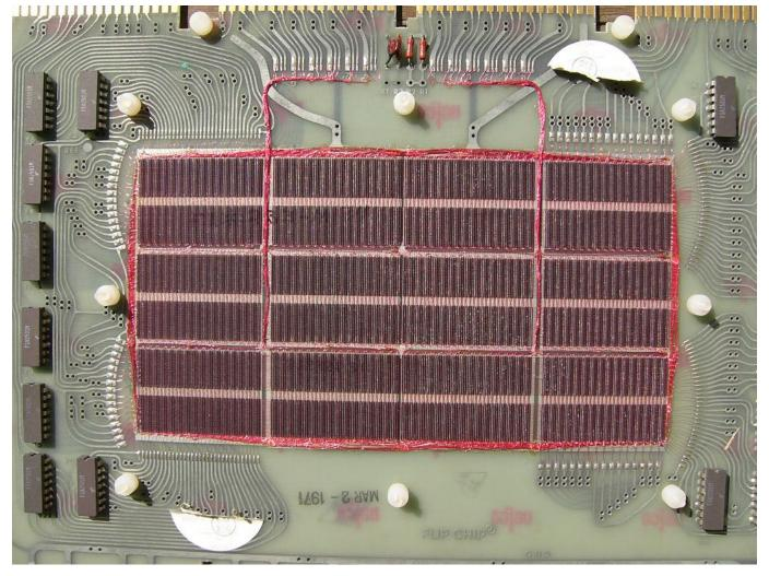
Figure 1: A 1970s core memory board.
