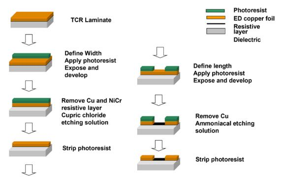
Figure 6: Thin-film resistor forming process sequence.
