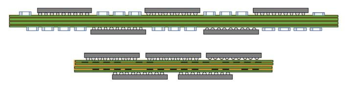
Figure 1: Comparing PCB area utilization of discrete surface-mounted resistors to that employing embedded thin-film resistors.
