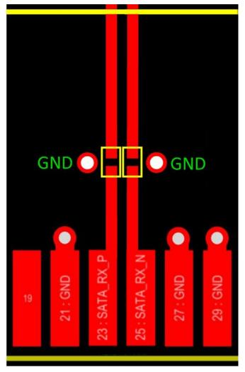
Figure 3: 200 µm trace with 01005 capacitors.
