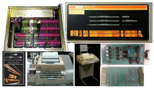
Figure 3: The digital PDP 8/L was the latest in 12-bit minicomputers. You had to manually toggle in the RIM Boot Loader with its front-panel switches so it could read a paper tape for the program from the ASR-35 teletypewriter. All the PCBs were single- and double-sided NPTHs with a wire-wrap backplane.
