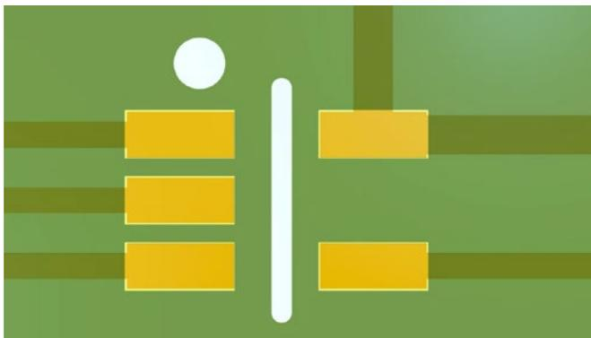
Figure 6: Clearance is just right and matches supplier capability.
