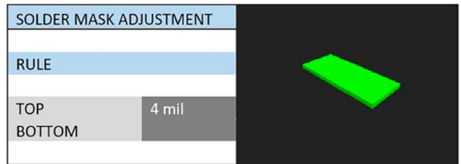
Figure 3: Setting the solder mask clearance values of your design tool.
