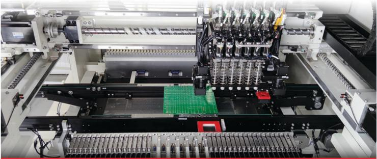
The MC889 Pick & Place machine sets new standards for precision, flexibility, and affordability. Places components from 01005 to 100 x 150 mm.
