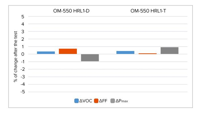
Figure 11: Damp heat and thermal cycling results of OM550 HRL1 assembled minipanels. D: 1000 h damp heat test. T: 200 cycles thermal cycling test.
