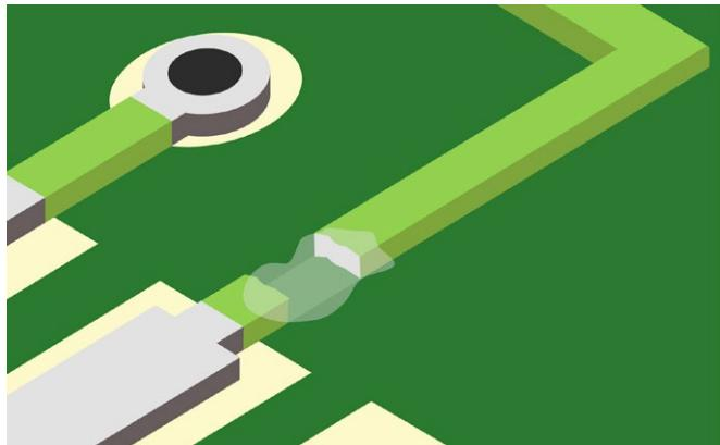
Figure 3: Fill in the gap of the trace cut using PCB repair epoxy.
