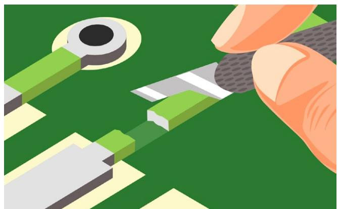
Figure 2: Use a sharp-edged knife to make the trace cuts.
