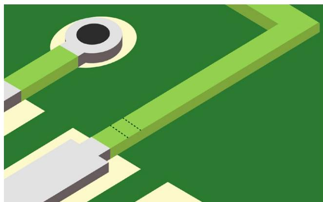
Figure 1: Determine the trace cut location.
