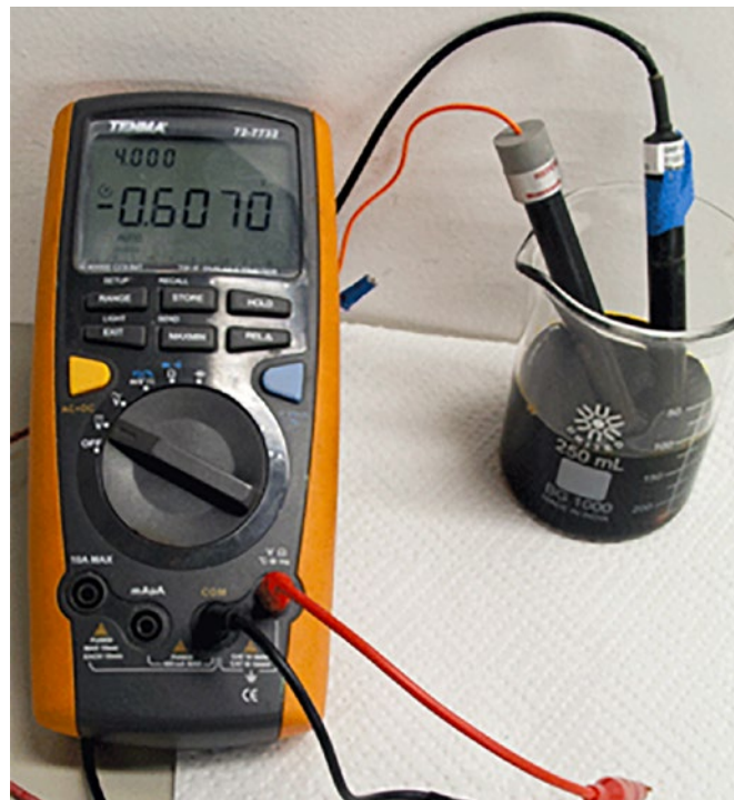
Figure 2: A basic ORP probe set-up for a beaker test.
