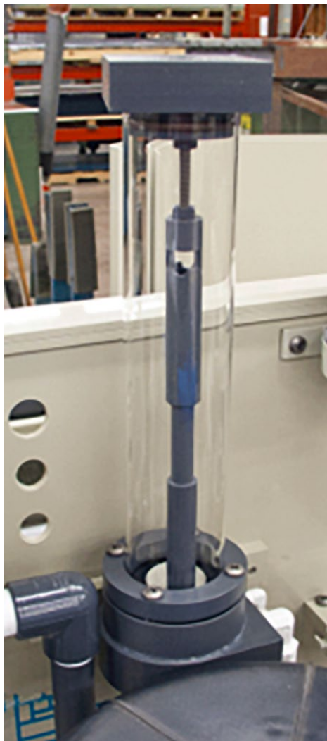
Figure 1: A standpipe (clear glass tube) on a piece of Chemcut equipment. This standpipe is equipped with a specific gravity controller (gray device in the middle of standpipe).
