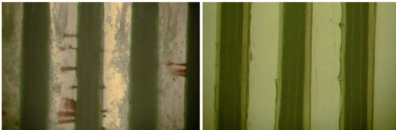
Figure 9: Observation under back-light: (left) dendrites with paste C; (right) no dendrite with paste D.
