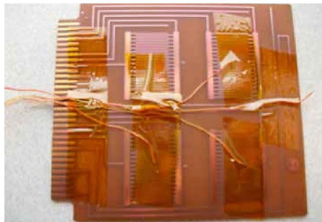
Figure 1: IPC-B-24 SIR test coupon with thermocouples attached.
