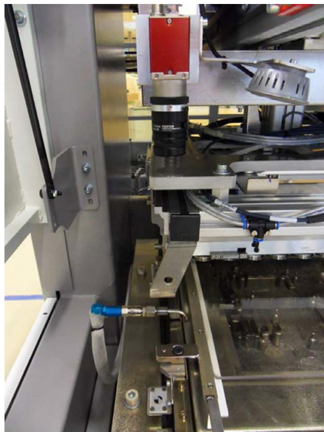
Figure 2: The camera mounted on the gripper verifies the position of the solder pot by checking the location of the fiducials.
