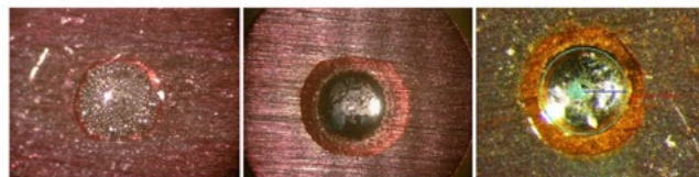
Figure 4: (l) Graping on 0.38 mm; (ctr) No graping on 0.76 mm; (r) Diameter 0.41 mm (initial 0.38 mm).
