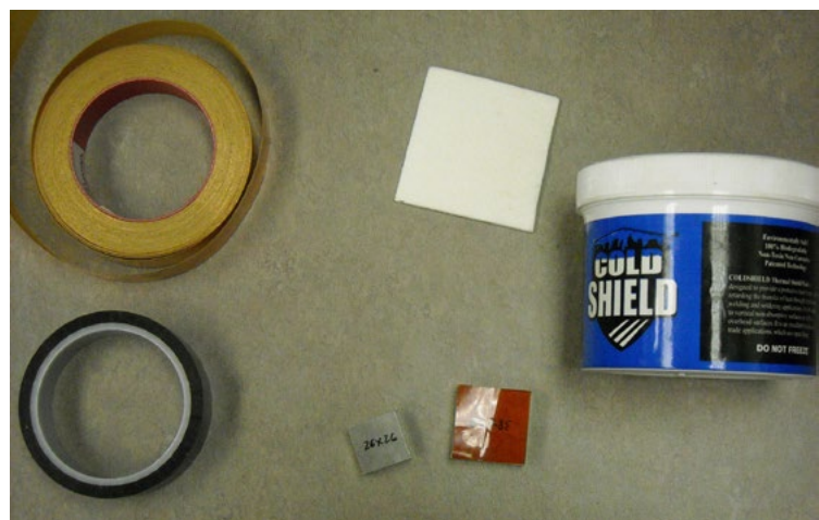
Figure 2: Materials used for shielding study, clockwise from upper left: copper tape, ceramic non-woven, clay/water, stainless steel and polyimide tape.
