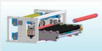
Easy removal of rollers with no tools (change of durometer rubber now possible)
