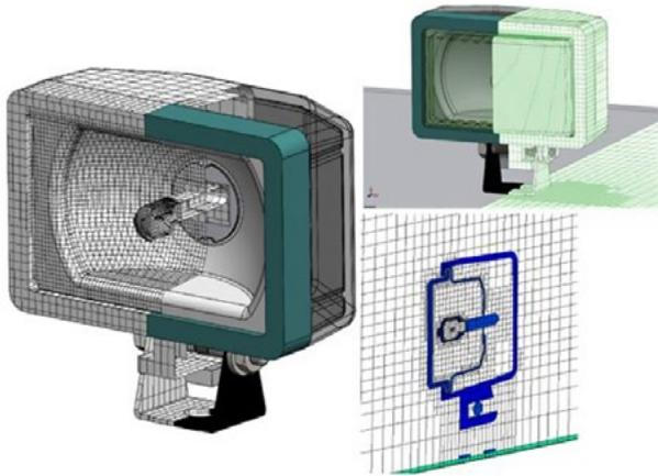
Figure 2: CFD Mesh needed to model the headlight in thermal simulations.
