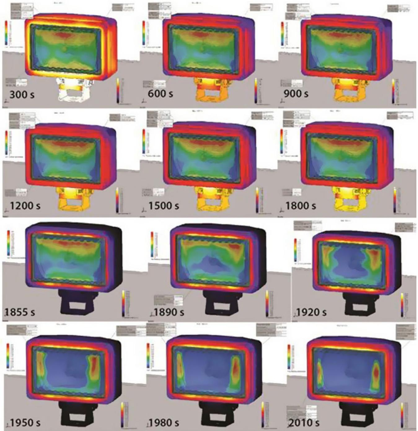
Figure 6: Simulation results of the changes in the condensation film thickness and contours that occurred over 30 minutes.
