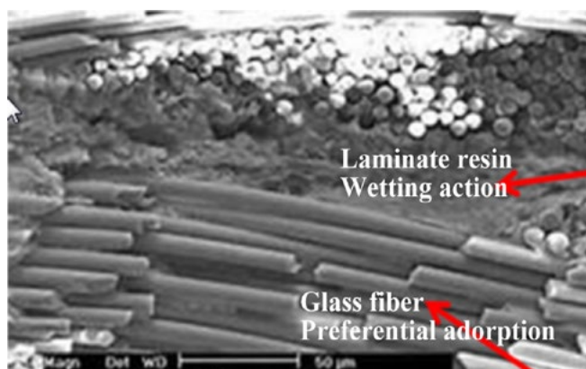
Figure 4: Typical rigid-flex substrate detail.
